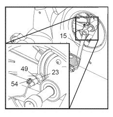
Slide the Reed Switch slightly closer to or away from the Magnet. Then, retighten the Screw. Turn the Left Crank Arm for a moment. Repeat until the console displays correct feedback. When the Reed Switch is correctly adjusted, reattach the left Pedal Guard (8) and the left Side Shield Cover (14).
