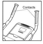
rate, hold the handgrip pulse sensor with your palms resting against the metal contacts. Avoid moving your hands or gripping the contacts tightly.
