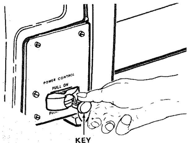
2. To turn Lathe ON . . . INSERT finger under switch lever and pull END of switch out.
