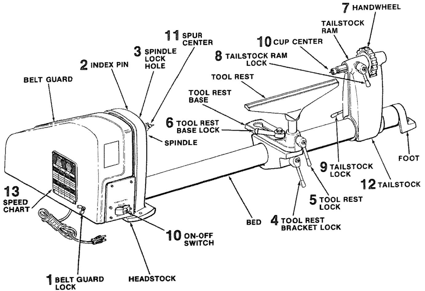
1. **BELT GUARD LOCK** ... Locks the hinged part of the guard during operation.
