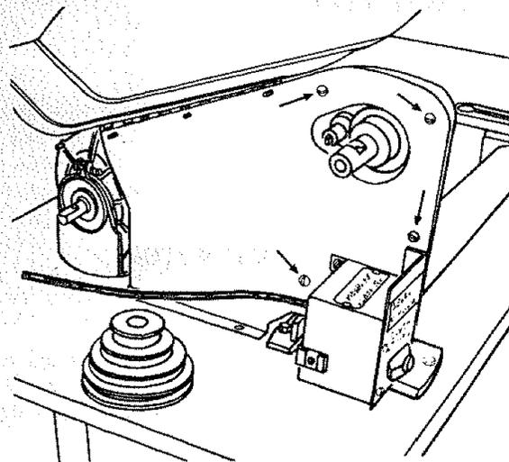
12. Place the headstock pulley onto the headstock shaft as shown. Position it so that the end of the pulley is flush with the end of the lathe spindle.
