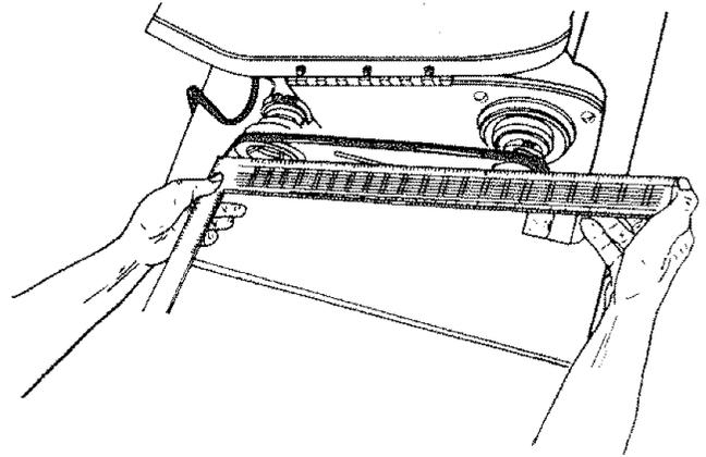
Attach the belt guard plate to the bench with the two screws. Make sure the plate is PARALLEL to the belt.
