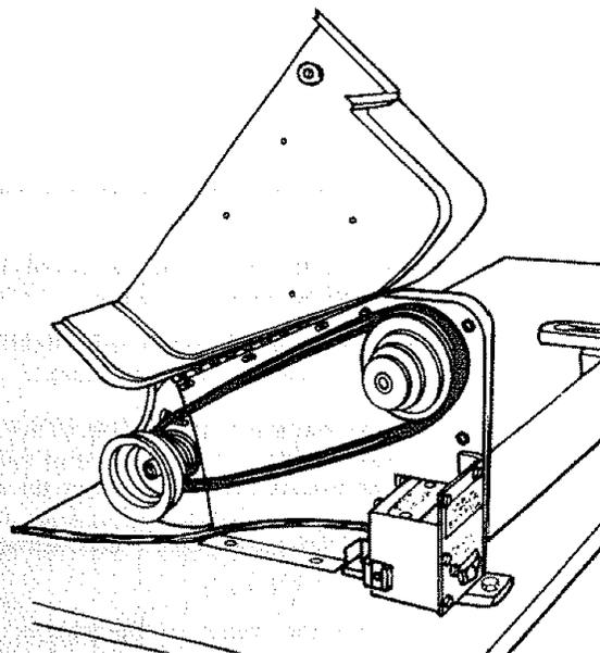
15. **NOTE:** When installing the pulley on a 1/2" diameter motor shaft, make sure that the adapter sleeve and 3/16" square key furnished with your motor are in place. Then tighten the setscrew with a 5/32" setscrew wrench.
