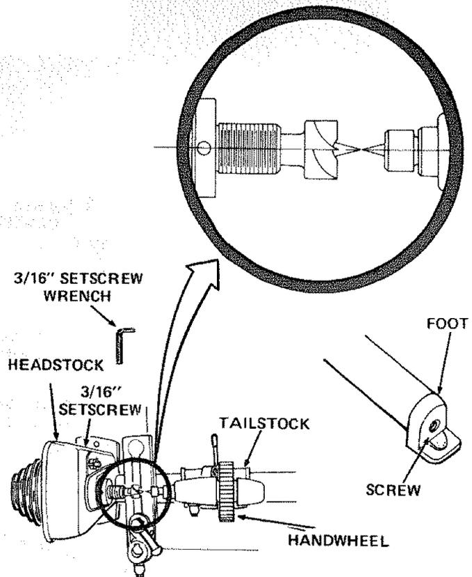
**12. TAILSTOCK** . . . supports the workpiece for spindle turning.
