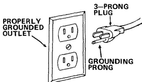
This power tool is equipped with a 3-conductor cord and grounding type plug which has a grounding prong, approved by Underwriters' Laboratories. The ground conductor has a green jacket and is attached to the tool housing at one end and to the ground prong in the attachment plug at the other end.
