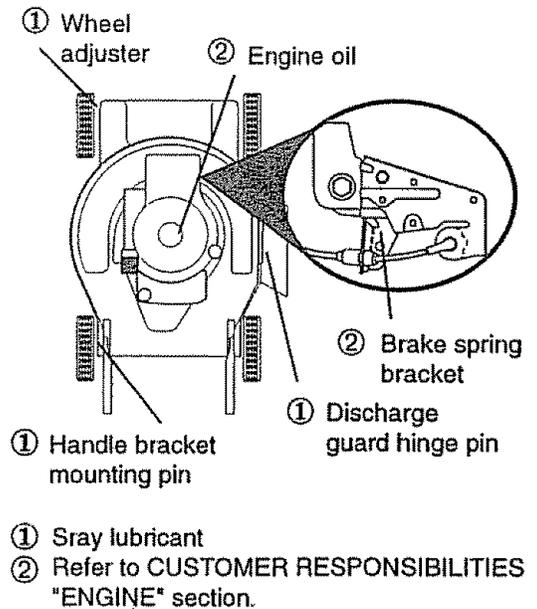
**IMPORTANT:** Do not oil or grease plastic wheel bearings. Viscous lubricants will attract dust and dirt that will shorten the life of the self lubricating bearings. If you feel they must be lubricated, use only a dry, powdered graphite type lubricant sparingly.
