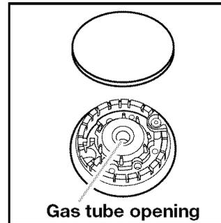
replace the burner cap. To replace the burner cap, make sure the alignment pins on the cap are properly aligned with the burner base.
