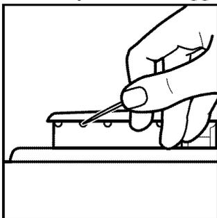
5. After cleaning the gas tube opening and ports, replace the burner cap.
