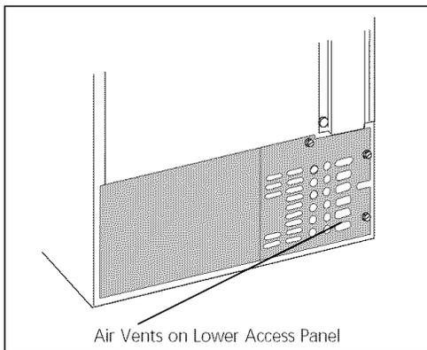
The air vents on the lower access panel at the rear of the refrigerator should be cleaned periodically. Clean the vents by using a vacuum cleaner with its dusting tool attachment. When moving the refrigerator, pull straight out. Do not shift the refrigerator from side to side as this may tear or gouge the floor covering. Be careful not to move the refrigerator beyond plumbing connections.
