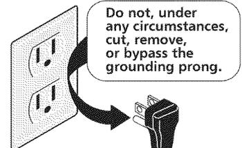
Power supply cord with 3-prong grounding plug
