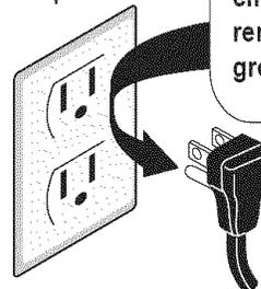
Power supply cord with 3-prong grounding plug
