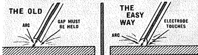
Special coating containing powdered iron forms a shell around wire core. Core burns back from outside coating to keep proper gap. Easiest arc welding method known.
