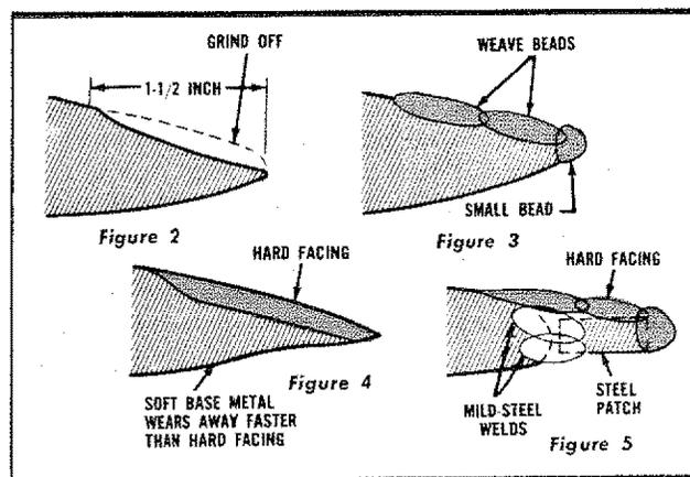
must be deposited along the edge to build it up (fig. 3). Make beads heaviest where the wear will be greatest, but avoid excessive build-up as the metal cannot be filed or machined. If shaping is required, heat the weld metal and forge it. Smoothing and sharpening can be accomplished by grinding.
