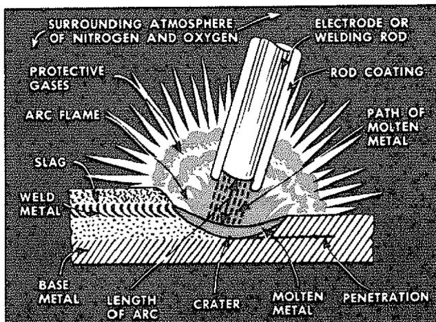
Arc Welding is the process of fusing two or more pieces of metal together to form one piece. It is accomplished by heating adjacent metal surfaces to the melting point with an electric arc, then adding a sufficient amount of molten metal to provide reinforcement and fill any vacant space between the parts being joined, as shown in the accompanying illustrations.
