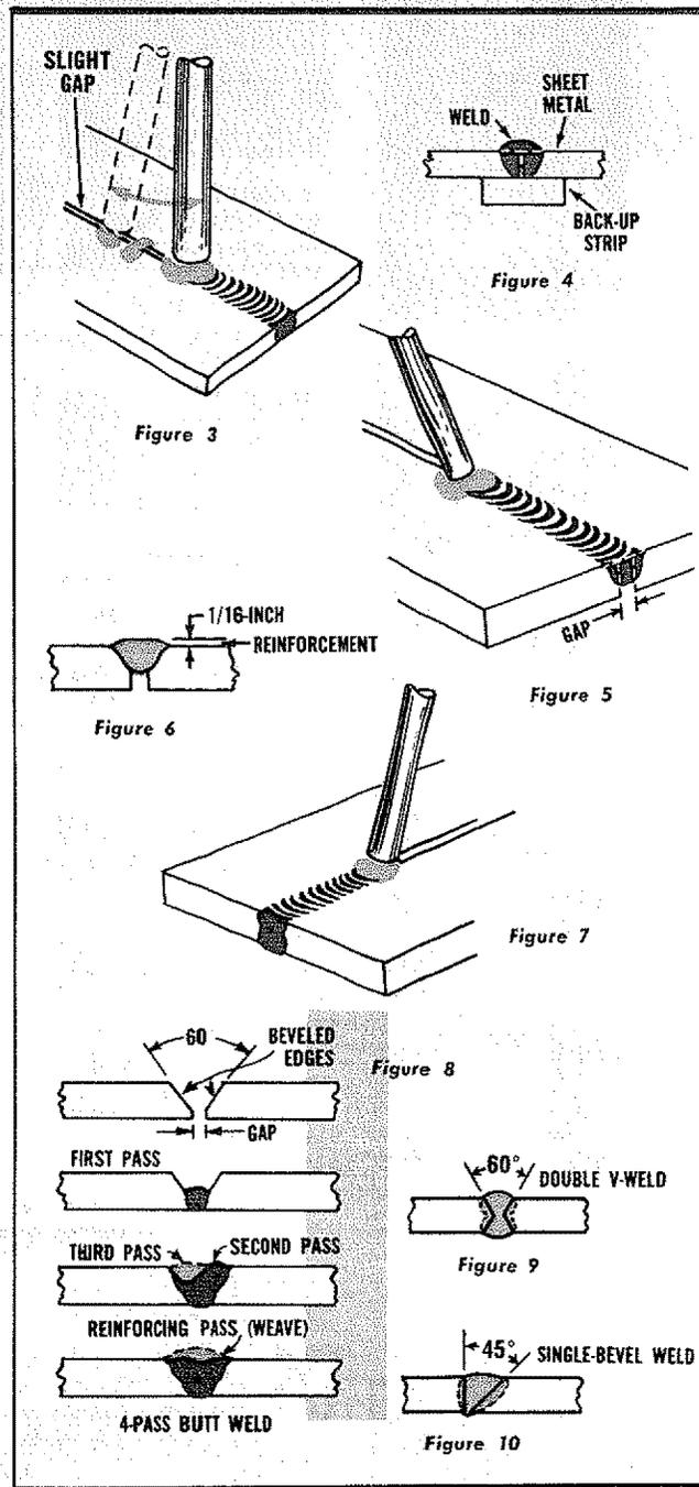
over and weld a similar bead on the other side (fig. 7). A higher welding current can be used on this side as there is no danger of burning through and fusion with the first bead will be assured.
