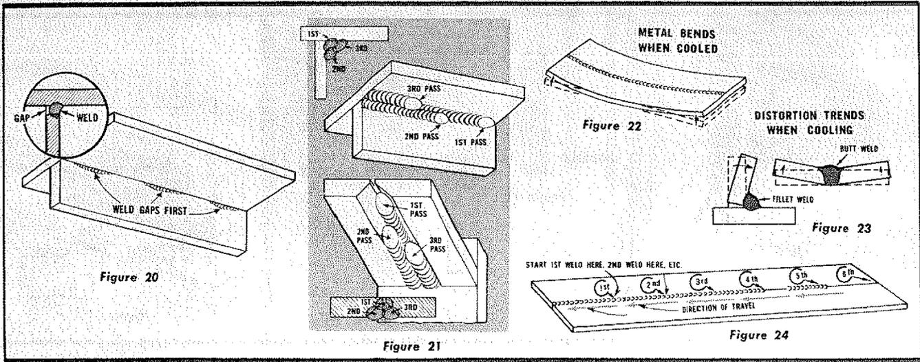
To simulate actual conditions tack-weld a piece with an irregular edge to another piece leaving numerous gaps along the joint. Use the whipping motion and deposit a fairly heavy bead, slowing down the rate of travel where the gaps are widest to build up a weld of uniform size throughout its length. If the gaps are rather wide, fill them first, clean off the slag and lay in a fillet weld the entire length of the joint (fig. 20).
