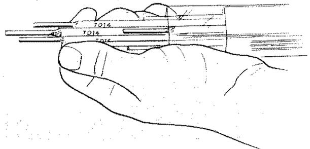
Now loosen the heat selector knob and move the pointer until the fractional number matching your electrode diameter appears in the pointer window.
