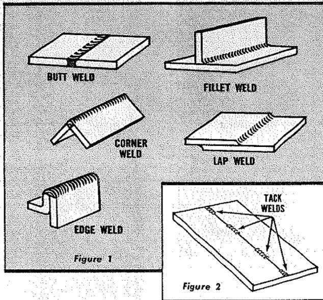
Flat welding includes all types of joints in which the weld is horizontal, and the electrode is fed down as in the practice welds of previous pages. The five types of joints in figure 1 can be welded in the flat position.
