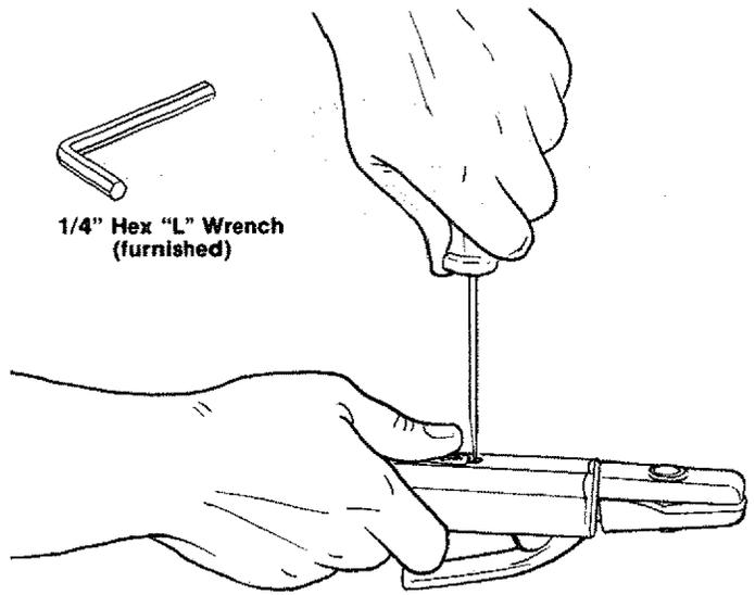
3. Using the sockethead wrench (supplied) back out the hex-head set screw, located near the end of electrode holder until the end of screw does not protrude into the wire socket in the end of holder.
