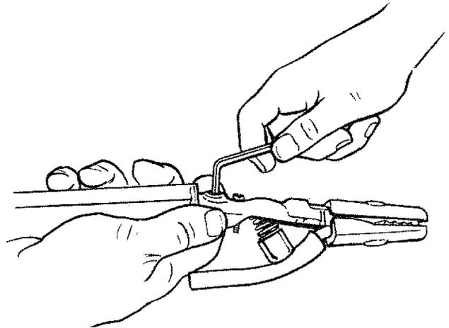
6. Slide the handle back into place on electrode holder and position it until the hole in handle is directly over the head of handle locking screw. Tighten the screw clockwise (↻) just enough to secure the handle on electrode holder.
