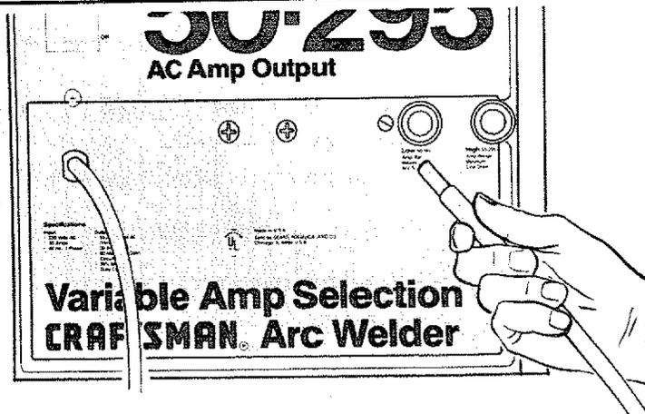
Connect the work clamp to the piece to be welded, (to complete the electrical circuit) or to the welding table itself provided it is metallic or will conduct electricity!
