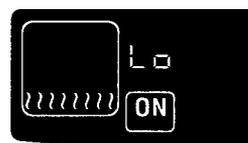
(example for Bake) ("Lo" is displayed after 5 seconds if oven temperature is below 170°F)
