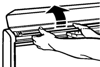
4. **Grasp** the fluorescent light tube at both ends. **Turn** the tube approximately 90° in either direction until both ends come out of the receptacles. **Replace** with a 20-watt cool-white fluorescent light tube.
