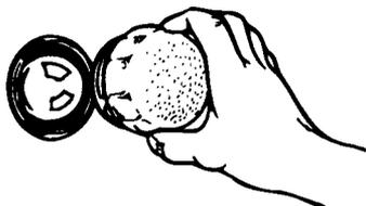
2. **Remove** the glass bulb cover in the back of the oven by screwing it out counter-clockwise.
