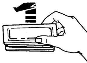
2. **Remove** glass light cover by grasping front edge of cover and pulling it away from the side wall of the oven.
