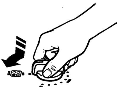
2. After the burner lights, turn the control knob to the desired setting.
