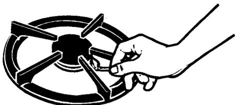
1. Hold a lit match near a burner and turn the control knob to the HI position.
