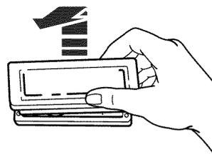
3. **Remove** glass light cover by grasping front edge of cover and pulling it away from the side wall of the oven.
