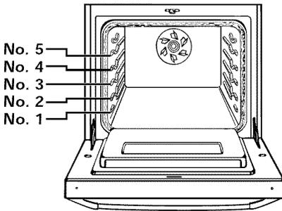
Your oven has three straight racks and five rack positions. Rack position 5 is the highest position, or farthest from the bottom of the oven. Rack position 1 is the lowest position, or closest to the bottom of the oven.
