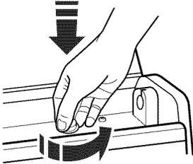
**To remove and replace the starter, first remove light tube. Push** starter in and **turn** approximately 90° counterclockwise. **Pull** starter out of recessed area. You can find replacement starters at stores that sell fluorescent light tubes.
