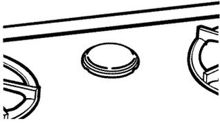
Hot air and moisture escape from the oven through a vent in the center rear of the cooktop. **Do not block the vent by using large pans or covers.** Poor baking/roasting and combustion can result.
