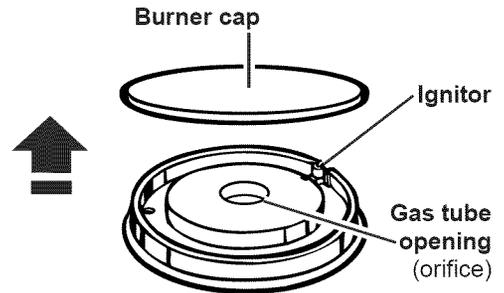
1. **Lift** the burner cap straight up from the burner base.
