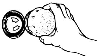
3. **Remove** the glass bulb cover in the back of the oven by turning it counterclockwise.
