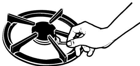
1. Hold a lit match near a burner and turn the control knob to the HI position.
