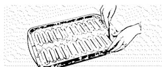
Cut slits in the foil just like the grid.
