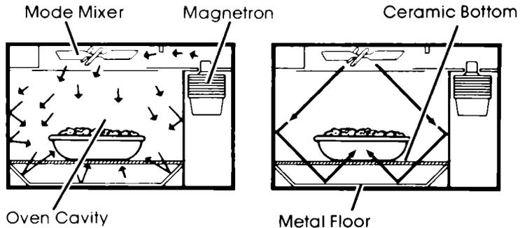
A magnetron in the microwave oven produces microwaves. The microwaves move into the oven where they are scattered or stirred by a mode mixer (like a fan). Microwaves bounce off metal oven walls and are absorbed by food.
