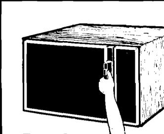
**DO NOT** attempt to operate this oven with the door open since open-door operation can result in harmful exposure to microwave energy. It is important not to defeat or tamper with the safety interlocks.
