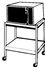
**2.** Put the oven on a cart, counter, table or shelf that is strong enough to hold the oven. **(The control side of the unit is the heavy side. Handling can be tricky.)**
