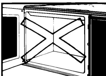
Starting a microwave oven when it's empty is not recommended. If you experiment, put a container of water in the oven.
