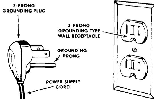
polarized 3-prong grounding plug. It must be plugged into a correct polarized mating 3-prong grounding type wall receptacle, properly installed and grounded in accordance with the National Electrical Code and local codes and ordinances. If a mating wall receptacle is not available or if you are not sure if the
