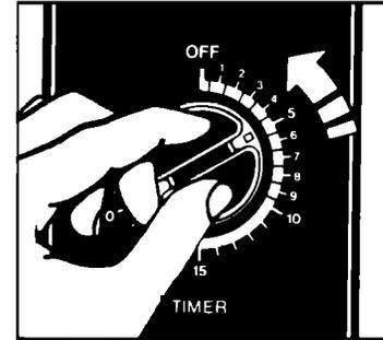
**To set the timer for less than 1 minute, turn Timer Knob past 1 minute, then to desired time.**
