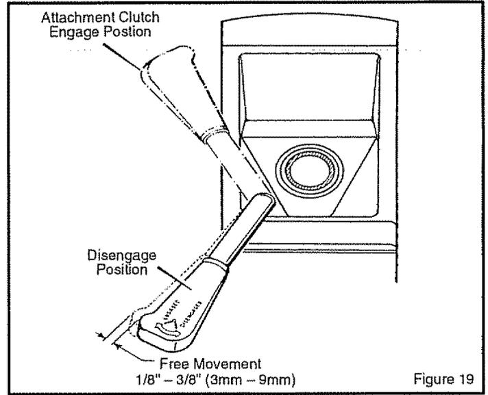
10. Attach the wire to the spark plug. Mow for a short distance and again check the operation of the **attachment clutch**.
