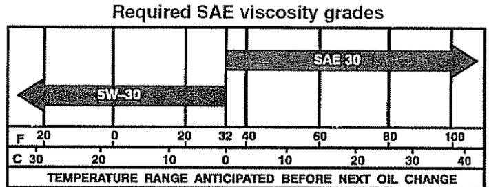
**NOTE:** Although multi-viscosity oils (5W30, 10W30, etc.) improve starting in cold weather, these multi-viscosity oils will result in increased oil consumption when used above 32° F. Check the engine oil level more frequently to avoid possible engine damage from running low on oil.
