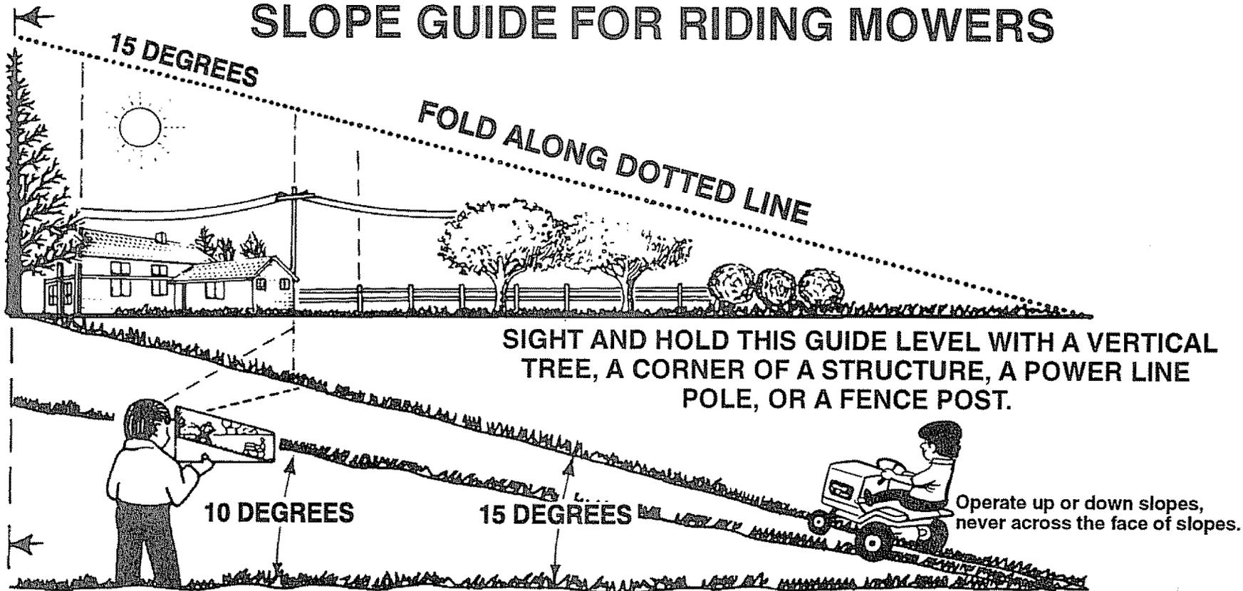
To determine if a slope is safe to mow: (1) disengage the blade(s), (2) put the unit in reverse, and (3) try to back straight up the slope. If you can back up the slope, it is generally safe to mow. However, if you do not feel safe, or if you are not completely sure, use this guide and do not mow a slope that is greater than 15 degrees. If the riding mower is used with a pull-behind attachment, do not operate the unit on a slope that is greater than 10 degrees.
