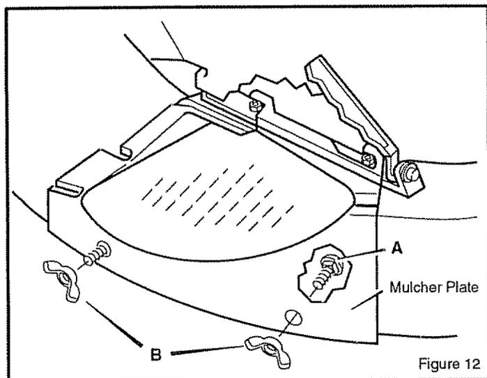
2. Slide the mulcher plate toward the front (Figure 13). Make sure the tabs on the mulcher plate are not locked behind the nuts.
