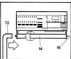
3. Align the lower end of the Side Rail (72) with the hole in the side of the treadmill Frame (58). Attach the Side Rail with a Side Rail Bolt (70), Formed Washer (71) Side Rail Washer (73) as shown. Tighten the Lock Knob (see step 1).
