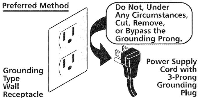
Where a standard two-prong wall receptacle is encountered, it is the personal responsibility and obligation of the customer to have it replaced with a properly grounded three-prong wall receptacle.
