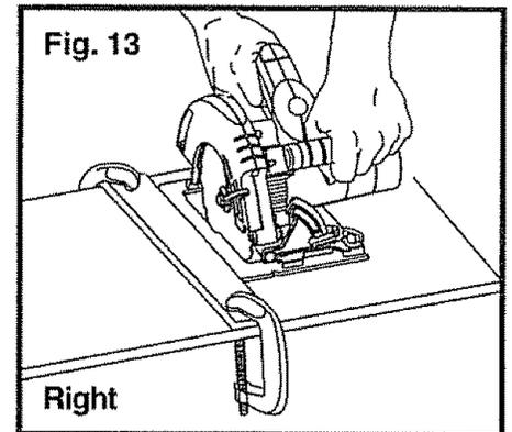
**⚠ DANGER:** When sawing through the workpiece, the lower blade guard does not cover the blade. The blade is exposed on the under side of the workpiece. **ALWAYS** keep your hands and fingers away from the cutting area. Any part of your body coming in contact with the moving blade will result in serious injury.
