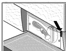
The cycle will continue when the power is back on. However, if the laundry should be removed, the loading door can be opened as described in the following:
