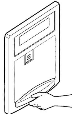
Tilt up the front of tray slightly and snap the ribs into the holes to replace the tray.
