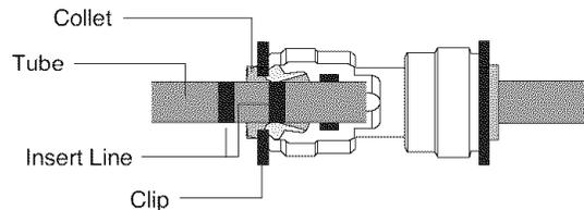
After inserting, pull the tube to ascertain that it is secure and assemble the clip.
