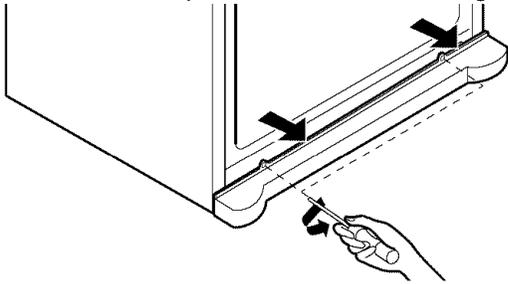
2. Turn the leveling leg clockwise to raise that side of the refrigerator or counterclockwise to lower it. It may take several turns of the leveling leg to adjust the tilt of the refrigerator.
