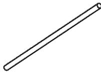
To determine how much tubing you need: measure the distance from the water valve on the back of the refrigerator to the water supply pipe. Then add 8 feet (2.4 m). Be sure there is sufficient extra tubing (about 8 feet [2.4 m] coiled into 3 turns of about 10" [25 cm] diameter) to allow the refrigerator to move out from the wall after installation.
