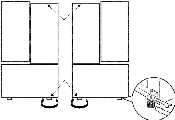
3. Open both doors again and check to make sure that they close easily. If not, tilt the refrigerator slightly more to the rear by turning both leveling legs clockwise. It may take several more turns, and you should turn both leveling legs the same amount.
