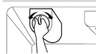
If you can't turn the filter from side to side, it isn't fully inserted. Push it in firmly and twist it into place. You will hear the snap when it clicks into place.
