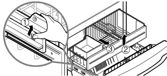
To install, reposition the gear part of rear left and right side of the drawer after pulling out both rails as much as possible, and gently push down both left and right side while checking the hook on the front part.
