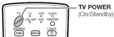
Press **POWER** on the TV, or **TV POWER** on the remote control unit to turn the power on.
