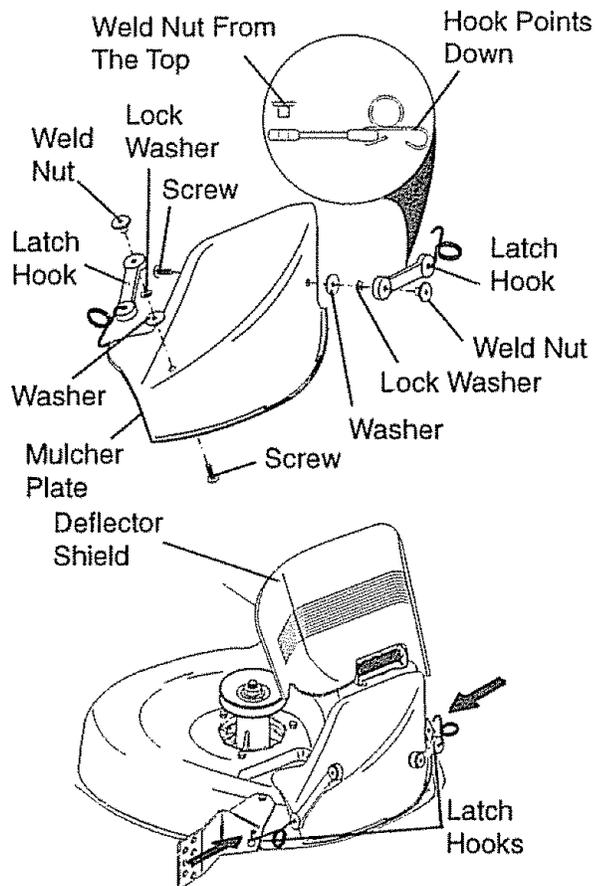
**CAUTION:** Do not remove discharge guard from mower. Raise and hold guard when attaching mulcher plate and allow it to rest on plate while in operation.
