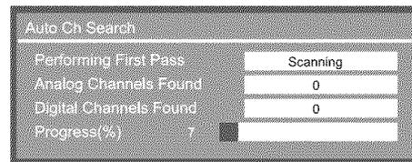
The TV will automatically cycle through all the antenna channels, and store all active channels in the channel memory. While the TV is cycling through the channels, the message "Progress(%)" appears a white bar to indicate the scanning status (as shown above).
