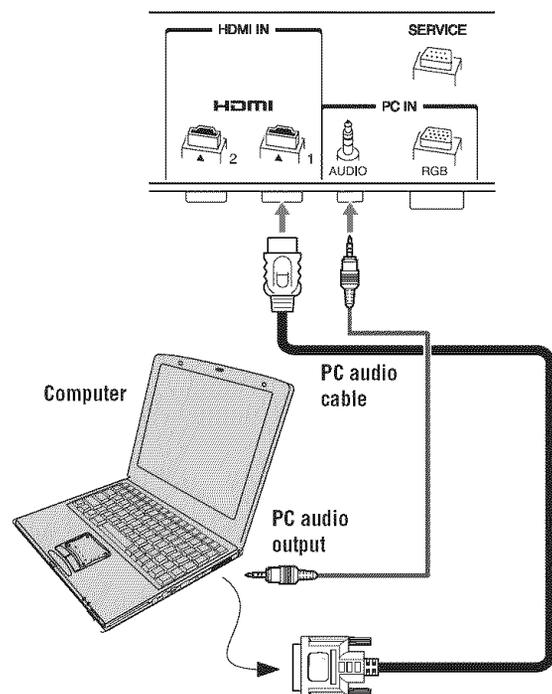
The HDMI 1 input can accept and display VGA, SVGA, XGA, 480i (60Hz), 480p (60Hz), 720p (60Hz), and 1080i (60Hz) signal formats. For detailed signal specifications, see page 49.
