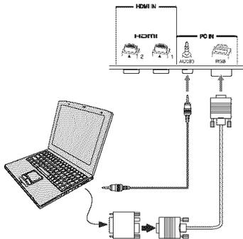
**Note:** Because the PC Audio input is shared with HDMI 1. If INPUT source is set to "HDMI 1," And the HDMI 1 signal is DVI format. This PC Audio input will apply for HDMI 1. (Also see item 2 on page 11.)
