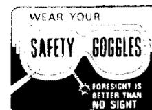
Any power miter saw can throw foreign objects into the eyes. This can result in permanent eye damage. Wear safety goggles (not glasses) that comply with ANSI Z87.1 (shown on package). Everyday eyeglasses have only impact resistant lenses. They are not safety glasses. Safety goggles are available at Sears retail stores. Glasses or goggles not in compliance with ANSI Z87.1 could seriously hurt you when they break
