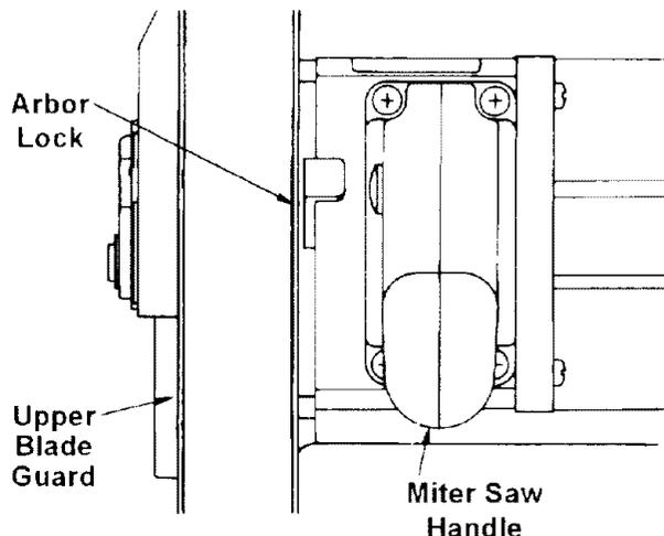
8. Install the outer blade collar, arbor washer and arbor screw. Press the arbor lock and turn the 1/2" wrench counter clockwise to secure the blade. Tighten arbor screw securely.
