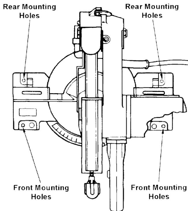
Place the saw in the desired location either on a work bench or the recommended leg set. The base of the saw has four holes to mount the miter saw (see illustration). If the saw is to be used in one location, fasten it to the work bench or leg set.
