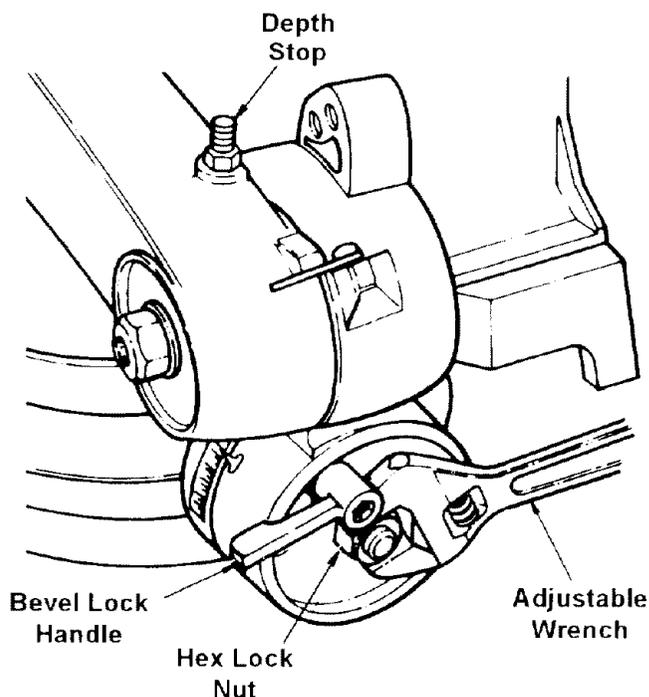
**WARNING: do not start the miter saw without checking for interference between the blade and the turn table structure. Damage could result to the blade if it strikes the turn table structure during operation of the saw.**
