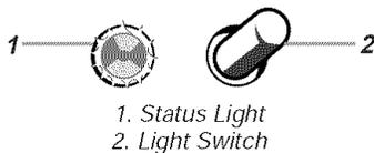
After changing the water filter cartridge, reset the water filter status light by pressing the **light switch** 5 times within 10 seconds. The status light will change from red to green when the system is reset.
