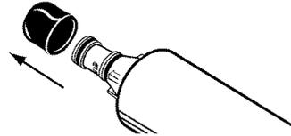
4. Slide the cartridge cap onto the new cartridge as shown above in Step 2.
