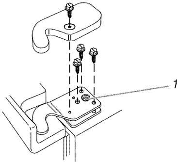
5. Remove bottom hinge, if necessary. Both bottom hinges have similar construction. **DO NOT REMOVE SCREW 1 AS SHOWN IN DIAGRAM.**
