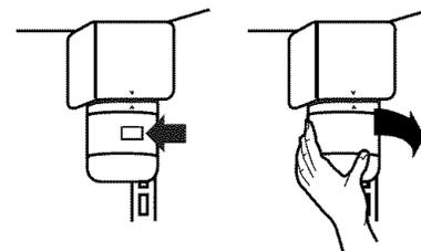
3. Line up the INSTALL mark on the water filter label with the indicator line that is molded into the filter mounting bracket cover. Push the cartridge into the filter mounting bracket. Twist the cartridge ¼ turn to the right to lock it into place. The REMOVE mark should be lined-up with the indicator line located on the front cover.
