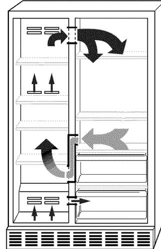
**Do not block any of these vents** with food such as soda, cereal, bread, etc. If the vents are blocked, airflow will be prevented and the temperature controls will not function properly.
