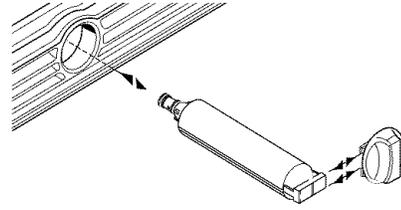
3. Take the new cartridge out of its packaging and remove protective cover from o-rings.
