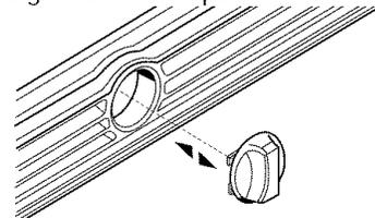
3. Rotate the cartridge cap to a horizontal position as shown in step 5.
