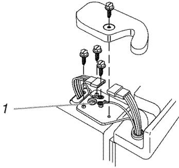
4. Disassemble right top hinge.
