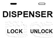
**NOTE:** The lock feature does not shut off power to the product, to the ice maker, or to the dispenser light. It simply deactivates the dispenser levers.
