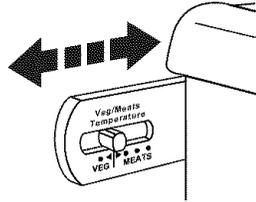
**IMPORTANT:** If food starts to freeze, move the control to the left (less cold). Remember to wait 24 hours between adjustments. Doing so gives the temperature of the food time to change.
