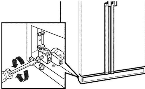
5. Open both doors again and check to make sure that they close as easily as you like. If not, tilt the refrigerator slightly more to the rear by turning both leveling screws to the right. It may take several more turns, and you should turn both leveling screws the same amount.
