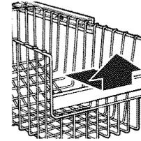
3. Replace the basket by positioning it on the side wall guide rails. Lift the basket front slightly while pushing it past the guide rail stops and slide basket in the rest of the way.
