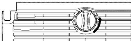
2. Remove the cartridge cap by sliding it off the end of the old cartridge. The cap will slide to the left or right. **DO NOT DISCARD THE CAP.**
