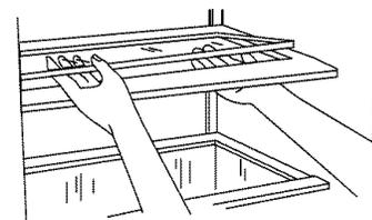
3. Replace back of meat drawer cover frame into supports on side walls of the refrigerator and lower the front of the cover frame into place.
