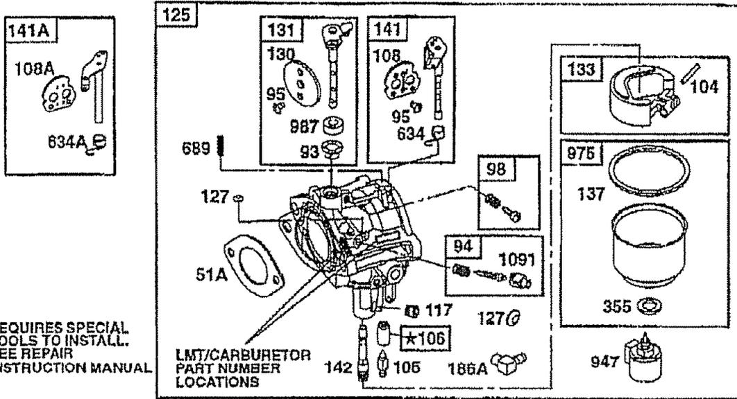
THIS CARBURETOR SERVICES BOTH CHOKE-A-MATIC AND MANUAL CHOKE SYSTEMS
