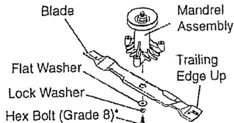
\*A Grade 8 heat treated bolt can be identified by six lines on the bolt head.
