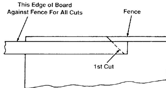
Turn Workpiece Over End For End...Keep Same Edge Against Fence When Making Successive Cuts.
