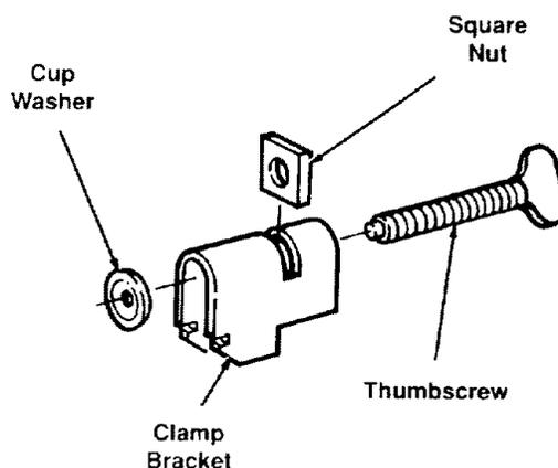
5. Tilt clamp bracket forward and snap into place in opening at rear of table support.
