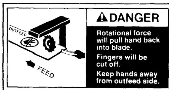
If you reach around the blade to the outfeed side when ripping, and try to hold down or pull the workpiece through to complete a cut, the rotational force of the blade will pull your hand back into the blade.
