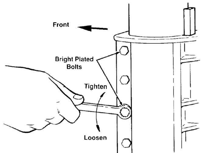
4. Now tighten the (2) 1/4 - 20 Gib socket cap screws until no noticeable rotational play exists between Column Tube and Column Support as shown in step 1.
