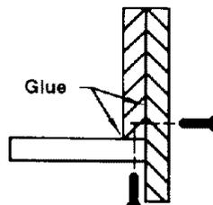
Use 2 screws in at least 2 equally spaced locations along fence (for a total of 4 screws)
