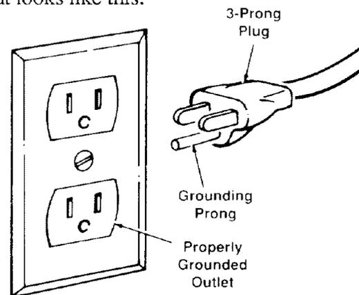
The power tool is equipped with a 3-conductor cord and grounding type plug listed by Underwriters' Laboratories. The ground conductor has a green jacket and is attached to the tool housing at one end and to the ground prong in the attachment plug at the other end.
