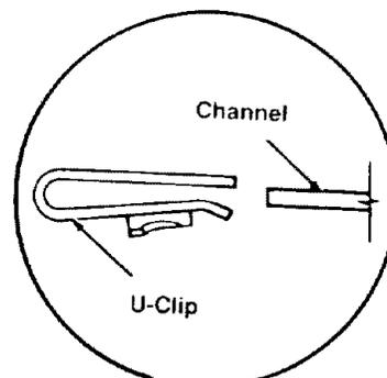
4. Place table, **top side up**, on saw so center counterbored hole lines up with hole in U-clip. **Note:** Table will extend over front edge of saw frame.
