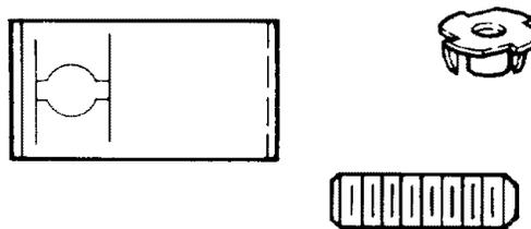
2. Identify top and bottom of table: top has counterbored holes. Place table **bottom side up** on solid surface. Hammer tee nut into leveling hole. (This hole is not counter-bored from the top).
