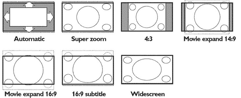
Super Zoom, Movie expand 14:9, Movie expand 16:9 and 16:9 subtitle makes the picture fill the screen as much as possible. It is recommended to press the cursor up/down key to adjust the picture position on the screen.
