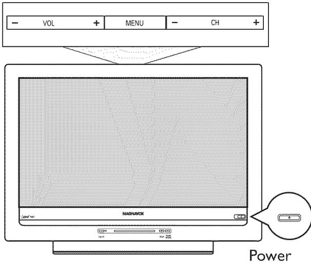
Should your remote be lost or broken you can still change some of the basic settings with the buttons on the top of your TV. Press the power switch
