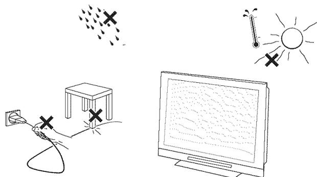
Place the TV on a solid surface. For ventilation, leave at least 4" to 6" free all around the TV. Do not place the TV on a carpet. To prevent any unsafe situations, no naked flame sources, such as lighted candles, should be placed in the vicinity. Avoid heat, direct sunlight and exposure to rain or water. The equipment shall not be exposed to dripping or splashing.
