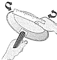
Pans should have flat bottoms. Check for flatness by rotating a ruler across the bottom. There should be no gaps between the pan and ruler.
