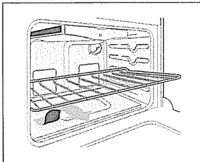
**To remove an oven rack**, pull the rack forward until it stops. Lift up front of rack and slide out. **To replace an oven rack**, fit the rack onto the guides on the oven walls. Tilt the front of the rack upward and slide the rack back into place.
