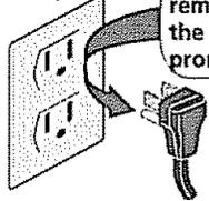
Power supply cord with 3-prong grounding plug
