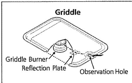
The hole in the griddle cover should be toward the backguard.
