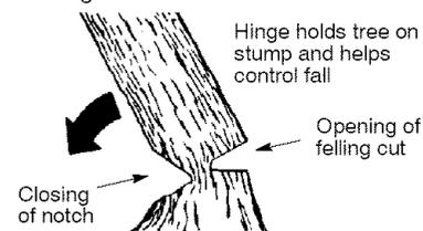
**NOTE:** Before felling cut is complete, use wedges to open the cut when necessary to control the direction of fall. To avoid kickback and chain damage, use wood or plastic wedges, but never steel or iron wedges.
