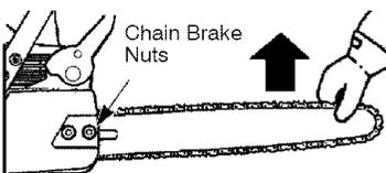
7. Use the screwdriver end of the bar tool to move chain around guide bar.
