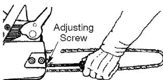
4. Using bar tool, roll chain around guide bar to ensure all links are in bar groove.
