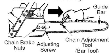
2. Loosen chain brake nuts until they are finger tight against the chain brake.
