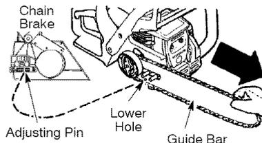
13. Install chain brake nuts and finger tighten only. Do not tighten any further at this point. Proceed to CHAIN ADJUSTMENT.
