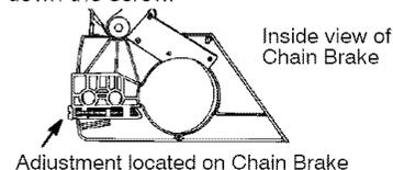
5. Turn adjusting screw by hand counterclockwise until adjusting pin just touches the stop.
