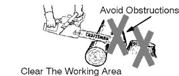
**⚠ WARNING:** Avoid kickback which can result in serious injury. **Kickback** is the backward, upward or sudden forward motion of the guide bar occurring when the saw chain near the upper tip of the guide bar contacts any object such as a log or branch, or when the wood closes in and pinches the saw chain in the cut. Contacting a foreign object in the wood can also result in loss of chain saw control.
