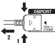
Press and hold both sides of the connector and then pull out the connector.
