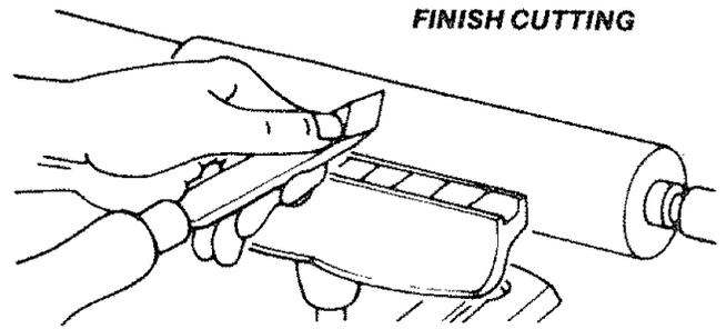
Finish cutting requires more control, with less force — and is better done with the palm of the tool-rest hand turned up. The wrist is still held down, and the side of the index finger acts as a guide along the rest. In this position, control of the chisel is shared by both hands, the fingers of the tool-rest hand being free to assist in positioning the tool.
