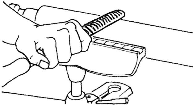
Finer finishes (similar to those produced by scraping) can be obtained by using files in the same manner. Various shape files can be used for shaping vees, beads, coves, etc. If pressed into the wood too hard, however, a file can burn the workpiece surface. Keep the file clean to keep it cutting uniformly. Files work best on hardwoods.
