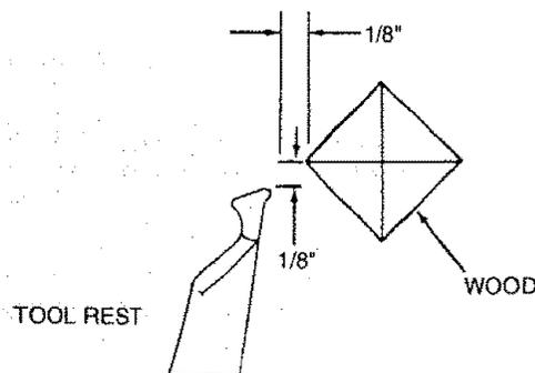
Look at the speed chart. Notice that a 2" square turning up to 18" long should run at 875 R.P.M. for "roughing". Move the V-belt on the pulleys to the slowest speed as outlined under "Changing Speeds" section.
