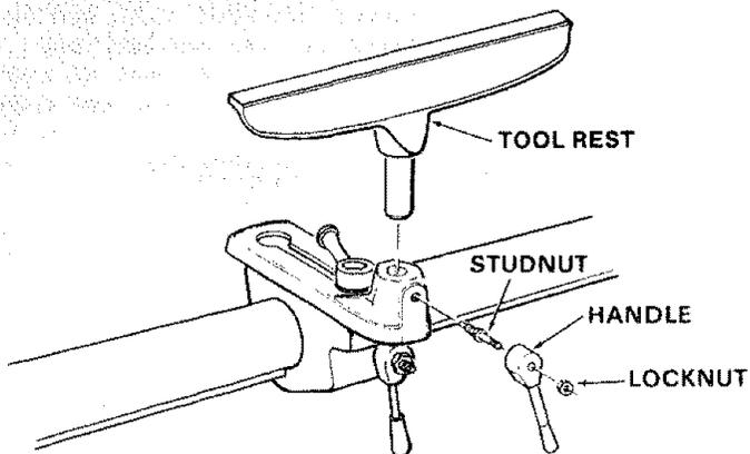
7. Slide tailstock assembly onto the tube and install tailstock ram spindle lock handle. Notice location of keyed way in spindle with studnut.
