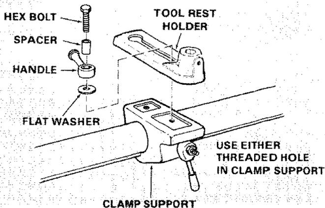
6. Set large tool rest in tool rest holder and install locking handle as shown.
