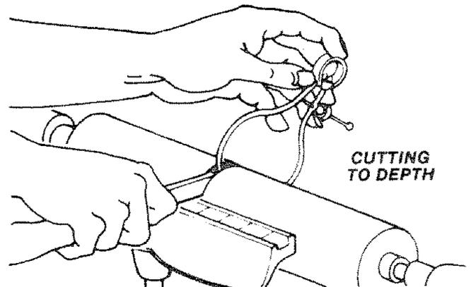
Many scraping operations and cutting to depth with the parting tool can be done with one hand. The chisel is grasped firmly, with the index finger on top to press it down against the rest — and is thrust straight into the work. Holding the tool thus leaves the other hand free to hold a pattern, calipers, etc., to check work progress.
