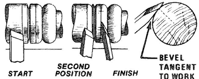
It is important that only the extreme heel should do the cutting. This means that the bottom edge of the bevel next to the vee must at all times be tangent to the arc of the bead being formed.
