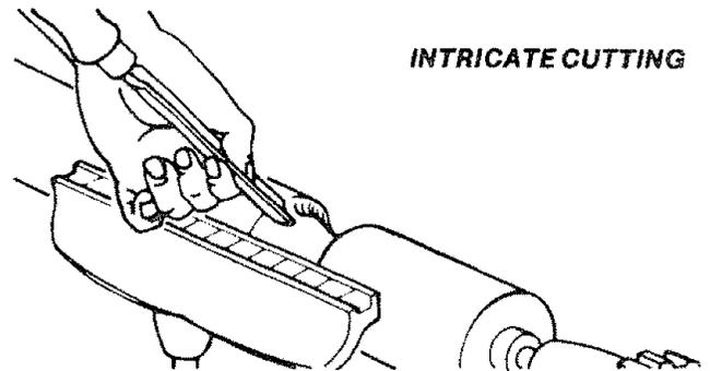
Intricate, delicate cutting requires extreme control, with practically no force. This is best accomplished by guiding the chisel with the fingers of the tool-rest hand. The hand is held palm up, with the wrist high — with the little finger placed against the rest to steady the hand. The chisel does not touch the rest; and the handle hand is completely secondary to the tool-rest hand.
