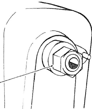
2. Find two points and a spur and cup center among the loose parts. To insert point into centers, place center between jaws of a vise. Do not tighten vise. Insert point into center and with a hammer and nail gently tap around the base of the point until secure.
