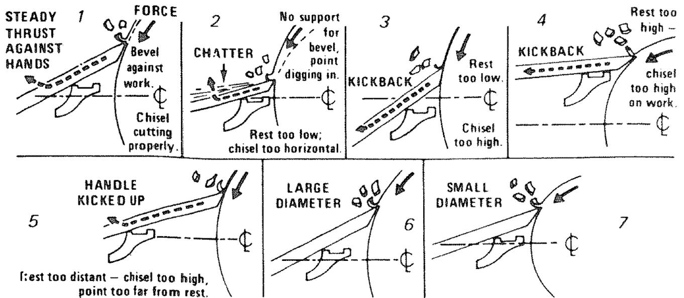
If the rest is placed too low, so that the chisel is held with the bevel out from the work (sketch 2), the cutting edge will continue to dig deeper into the work. It will dig in until the "bite" becomes so deep that your hands have difficulty holding the chisel — then the improperly supported chisel will begin to bounce, or chatter, against the workpiece.
