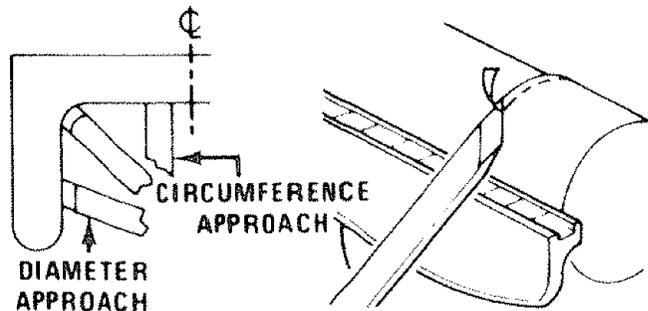
Either a cutting or scraping action can be used when the approach is toward a circumference — the shaving is removed like a peeling from a potato. Scraping, only, can be used when the approach is toward a diameter. The reason is obvious when you consider that faceplate turning practically always requires removal of wood across the grain. Wood does not peel easily across the grain, and attempts to use cutting methods will likely result in damage to the work and throwing of the chisel by the work.
