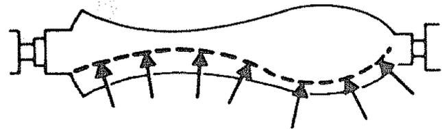
CHISEL INCLINED IN DIRECTION OF CUT
