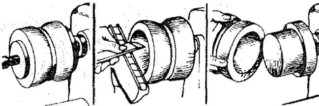
After making a recess at least 1/2 of the way through the workpiece, and finishing this on the inside, remove the workpiece from the lathe. Now mount a short length of softwood stock on the screw center and turn this down to form a dowel that will be a tight press (not driving) fit inside the recessed end of the cylinder. Mount the cylinder on this wooden chuck, and recess the unworked end deep enough to form a perfect hole through the entire cylinder.
