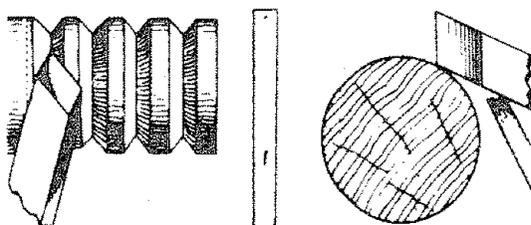
When the heel is used, the skew is rotated down into the work, using the rest as a pivot. Otherwise, cutting position and sequence of cuts is the same. As when using the toe, it is important that cutting be done only by extreme end of cutting edge.
