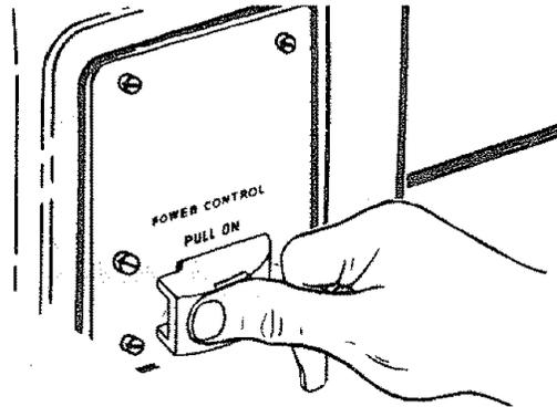
4. To lock switch in OFF position . . . HOLD switch IN with one hand, REMOVE key with other hand.
