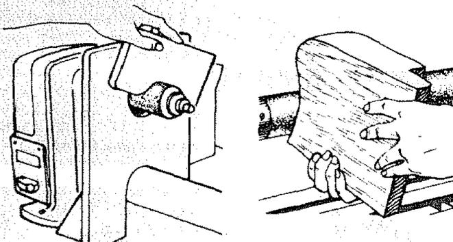
The drum is used mainly for sanding the edges of curved work. The squareness of the edge of the work can be best retained by using a simple form of vertical fence, as shown.
