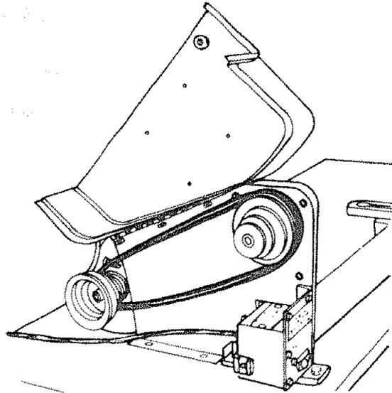
14. Place a straightedge such as a piece of wood, metal or framing square across the pulleys to see if they are in line with each other. If they are, tighten the other two motor mounting bolts. If they are not in line, loosen the two motor bolts and move the motor sideways . . . tighten the bolts.
