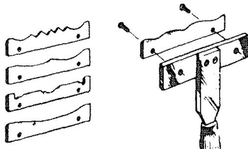
When a number of identical pieces are to be produced, all having a distinctive surface pattern, preformed tools will speed the work and assure uniformity. Patterns like those illustrated can be created by grinding thin (.020 to .010) gauge aluminum strips. A holder, like the one shown, can then be used to support any one of your prepared strips—and guide it against the workpiece.
