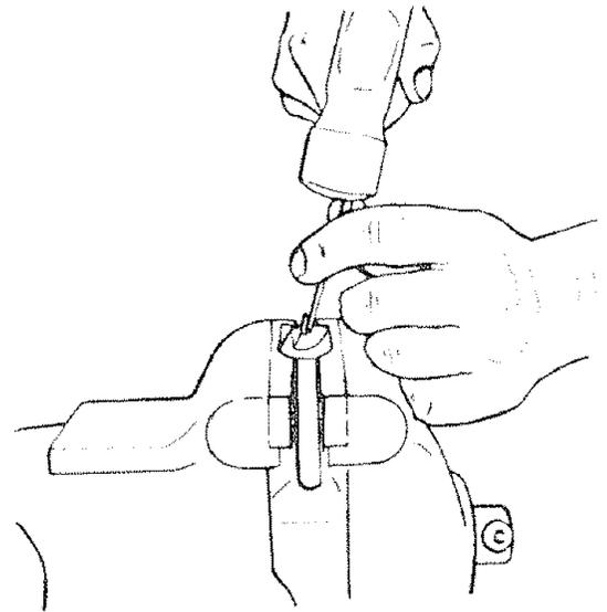
3. Insert spur center into head stock spindle and cup center into tailstock ram. **NOTE:** Do not drive or hammer centers into spindle or ram as removal may be difficult. Use a soft hammer or block of wood and give them a gentle tap.
