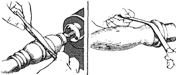
Turnings should be sanded with the lathe running in second lowest speed. A large sheet of sandpaper is useful for smoothing cylinders. All other sanding operations are done with a narrow strip of abrasive paper. The best finishing grit is 3/0 for softwoods, 4/0 for hardwoods.
