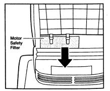
If the foam Motor Safety Filter located at the base of the bag cavity is dirty, remove it by pulling forward.
