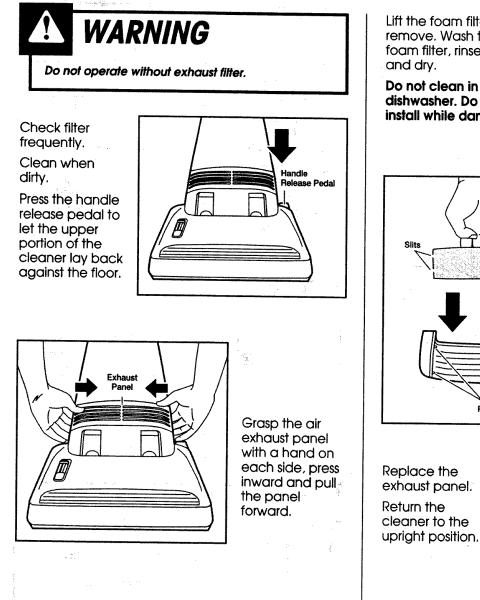
Lift the foam filter to remove. Wash the foam filter, rinse
