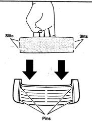
Replace the dry foam filter, carefully positioning it so the slits fit around the four raised pins.
