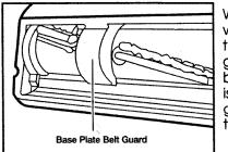
When brushes are worn to the level of the base plate belt guard or when the back-up beater bar is chipped or gouged, replace the brushes.
