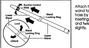
Attach the wand to the and twisting
