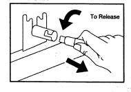
Pull the light bulb to remove.
