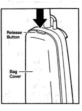
Pull the bag cover forward. Remove and lay aside.
