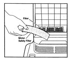
Check the filter located below the foam filter. If it is dirty, wipe it with a clean, dry cloth.
