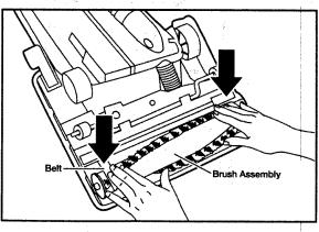
Press firmly, checking to see that each end is completely inserted.
