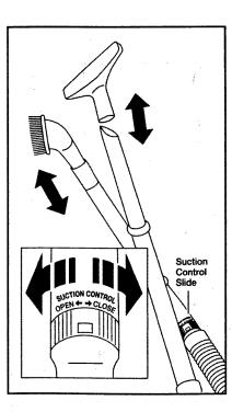
When using the dusting brush or the upholstery tool, they may be attached directly to the wand or placed on the end of the crevice tool.
