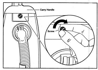
Using a screwdriver, tighten the screw.
