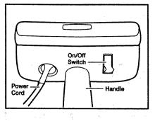
To start the vacuum cleaner, put the switch on the top of the body in the ON position. To stop the vacuum cleaner, put the switch in the OFF position.
