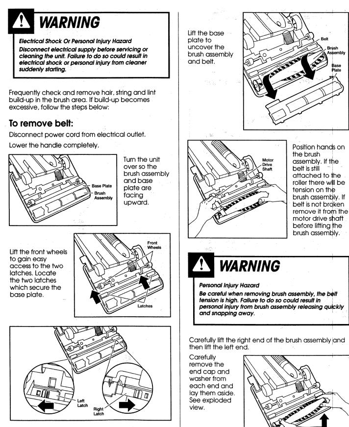
To unlock the base plate, slide the left latch to the left and the right latch to the right.
