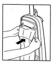
Position the bag cover so its positioning tab fits into the body positioning tab slot.
