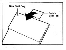
Fold the safety seal tab on the new bag away from the opening that fits on the dirt tube.
