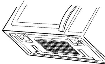
2. Remove the bulb cover mounting screws.
