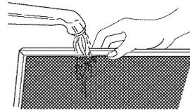
3. To reinstall the filter, slide it into the side slot, then push up and toward oven center to lock.
