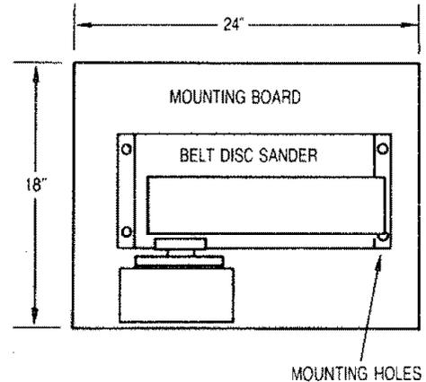
2. Substitute 5/16" flat head bolts for mounting bolts (NOT INCLUDED). Bolt length should be 1-1/2" plus the thickness of the mounting board.
