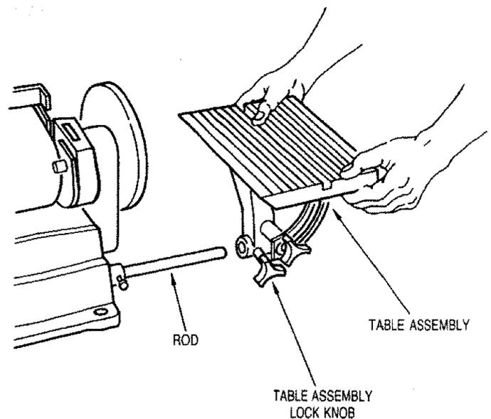
7. To adjust table so it is parallel to sanding surface, locate two allen head set screws on bottom side of the table.
