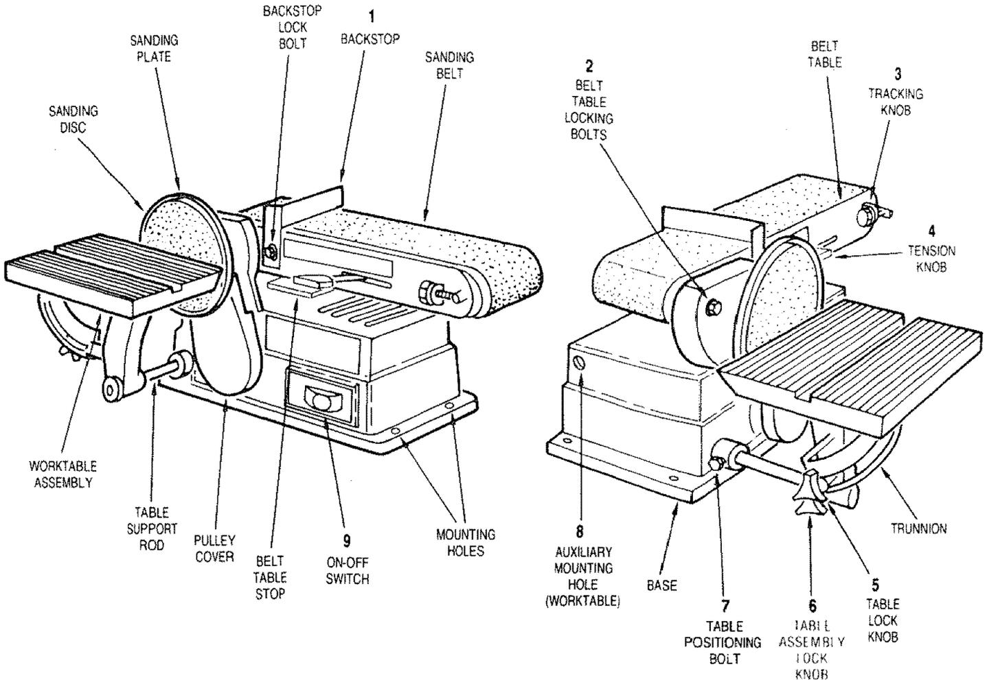
1. Backstop . . . Supports the workpiece on the sanding belt.
