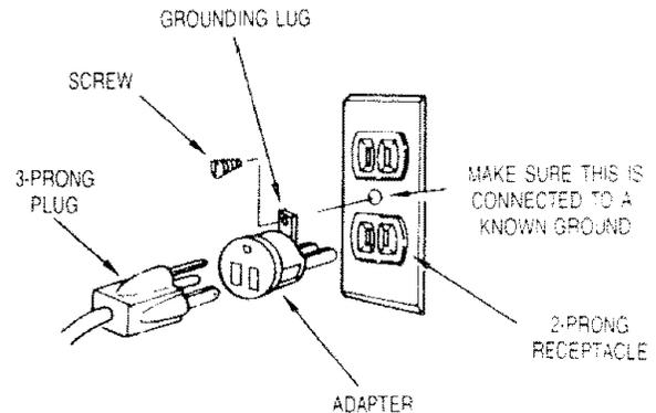
An adapter as shown above is available for connecting plugs to 2-prong receptacles.
