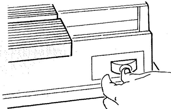
4. To lock switch in OFF position . . . hold switch IN with one hand . . . REMOVE key with other hand.
