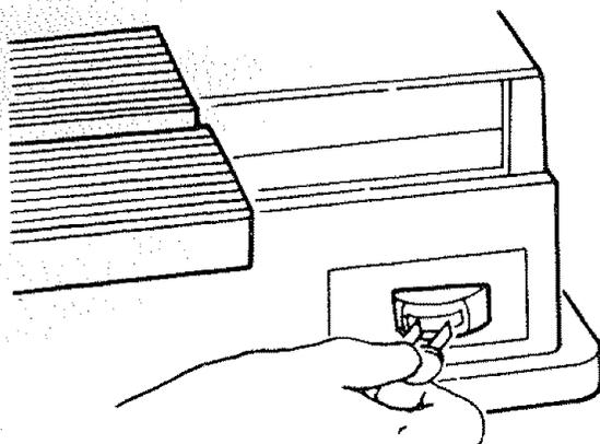
2. Insert finger under switch lever and pull end of switch out.
