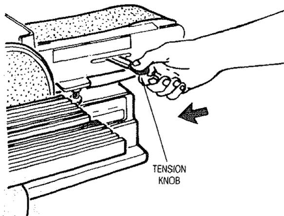
5. If the sanding belt moves toward the disc, turn the tracking knob counterclockwise 1/4 turn.
