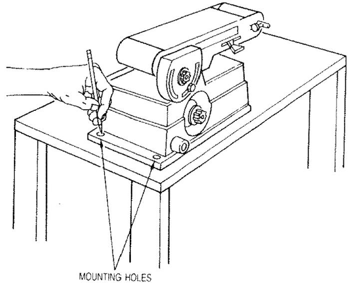
5. Insert four 5/16" bolts through the mounting holes and through the drilled holes in the workbench.
