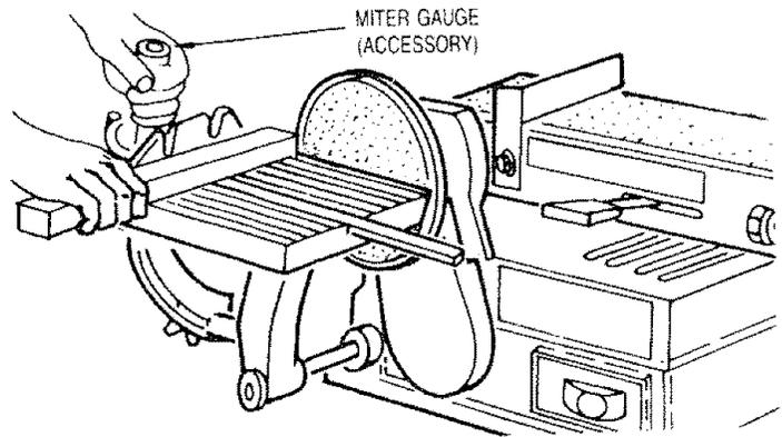
**NOTE:** Use a combination square to square the miter gauge to the face of the disc (combination square must be "true" — See Start of Assembly section on page 6 for checking method). If it is not square, loosen the miter gauge knob and move the miter gauge slightly until it is square. Without moving the miter gauge, tighten the knob securely.
