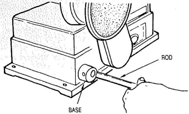
3. Install bolt in base (align a flat side of rod to bolt) and tighten with 1/2 inch wrench.
