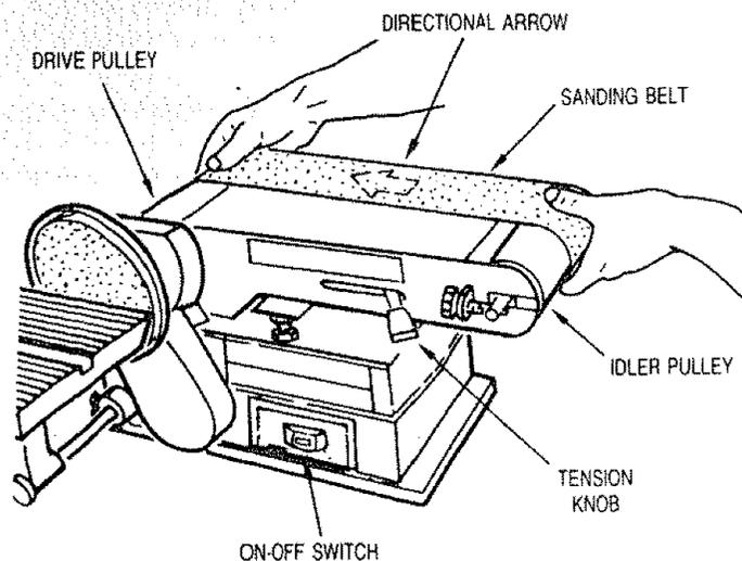
3. Slide tension knob to the left to apply belt tension.
