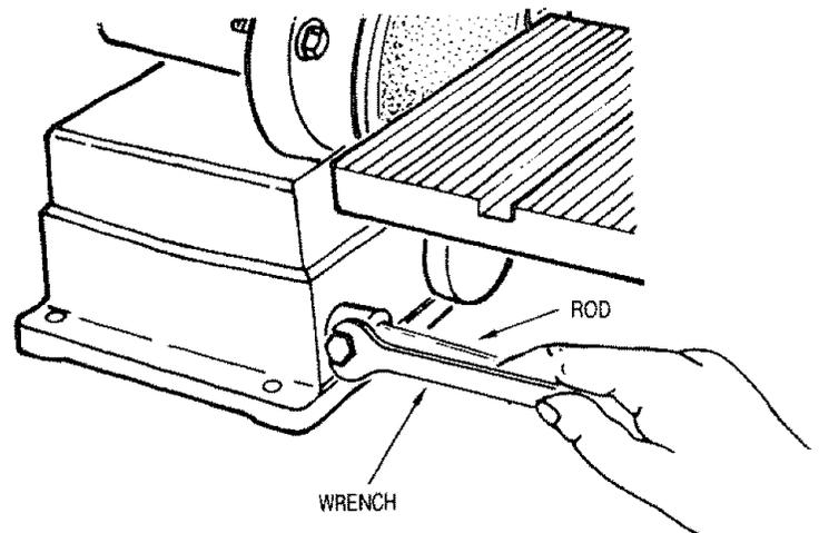
4. Slide table assembly onto rod.
