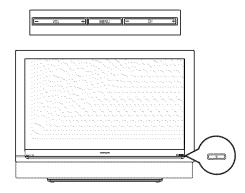
Should your remote be lost or broken you can still change some of the basic settings with the buttons on the top of your TV. Press the power switch  $\Phi$  to switch the TV on.
