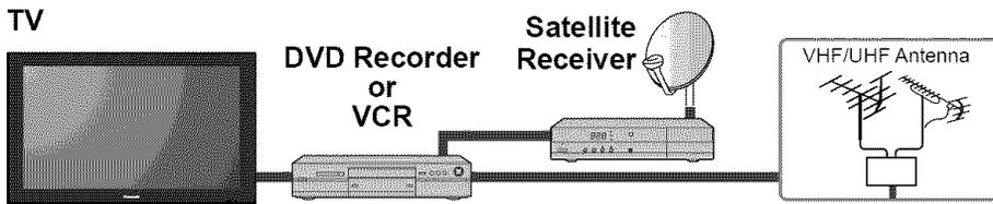
You can enjoy high-definition programming by subscribing to high-definition satellite service. Connection can be done with the use of HDMI or Component Video cable.
