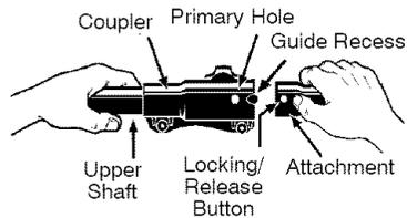
**WARNING:** Make sure the locking/release button is locked in the primary hole and the knob is securely tightened before operating the unit. All attachments are designed to be used in the primary hole unless otherwise stated in the applicable attachment op-
