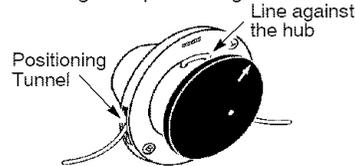
6. Correctly installed line will be the same length on both ends.
