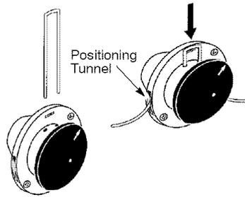
5. Pull the line and make sure the line is against the hub and extended full through the positioning tunnels.
