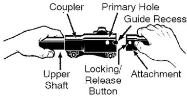
**WARNING:** Make sure the locking/release button is locked in the primary hole and the knob is securely tightened before operating the unit. All attachments are designed to be used in the primary hole unless otherwise stated in the applicable attachment operator's manual. Using the wrong hole could lead to serious injury or damage to the unit.
