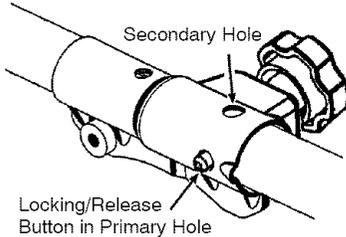
For optional attachments, see the ASSEMBLY section of the applicable attachment operator's manual.
