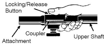
3. While securely holding the engine and upper shaft, pull the attachment straight out of the coupler.
