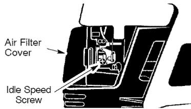
**⚠ WARNING:** Recheck the idle speed after each adjustment. The trimmer head must not move or spin at idle speed to avoid serious injury to the operator or others.
