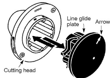
**NOTE:** Line glide plate must be reinstalled in cutting head before inserting new line.
