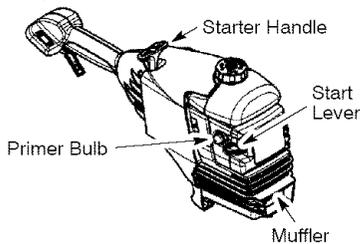
5. This unit has the Sim-pul™ starting system. You do not have to pull the starter rope handle sharply or briskly. Pull starter rope handle with a controlled and steady motion until engine starts and runs.
