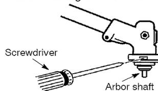
3. While holding the screwdriver in position, remove trimmer head by turning clockwise.
