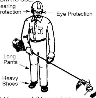
**WARNING:** Always wear eye protection and hearing protection. Never lean over the trimmer head. Rocks or debris can ricochet or be thrown into eyes and face and cause blindness or other serious injury.
