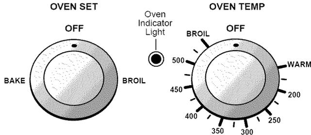
The **OVEN SET** knob determines the type of oven operation. Turn this knob to the desired setting. The oven will not operate if the **OVEN SET** knob is left in the OFF position.
