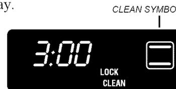
5. About one hour after the clean cycle ends, the LOCK indicator word will turn off. The oven door can be opened.
