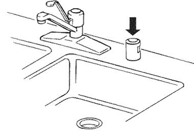
The drain air gap is usually located on top of the sink or countertop near the dishwasher. To order a drain air gap call your local dealer, or in the U.S.A., call the Customer Interaction Center and ask for Part Number 300096.
