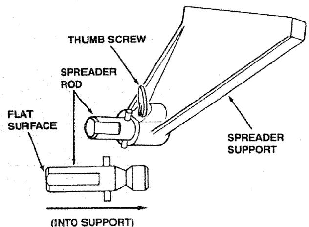
7. Slide SPREADER ROD into BLADE GUARD SUPPORT until end of ROD is even with edge of SUPPORT...Tighten Hex Head Screw in support.
