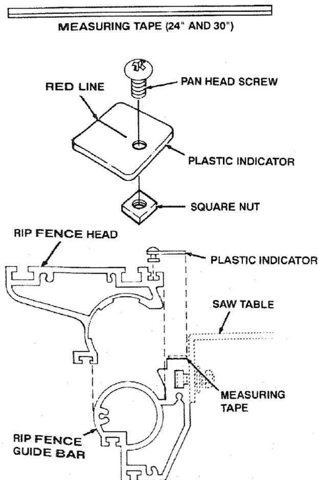
8. Find the "0" inch mark on the end of the 30" long right measuring tape. Slide this end of the measuring tape under the right side of the indicator and push tape along top surface of rip fence guide bar.
