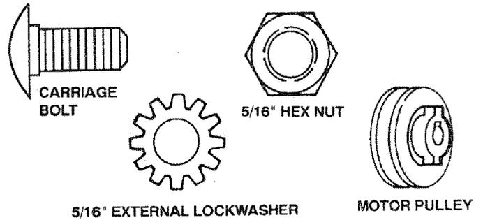
2. Place motor on MOTOR BASE, insert bolts through holes in base...then through the motor. Install lockwashers and nuts.
