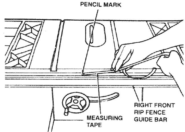
**NOTE:** If extreme accuracy is required when ripping, you should not use this method to position the fence. Instead, use a precision measuring instrument to set the rip fence the exact distance away from the blade.
