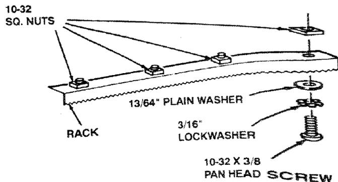
3. Install the other rack from the right end in a similar manner as described in #2, sliding rack against left rack. Tighten all screws.
