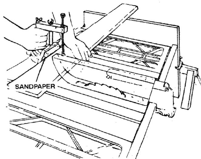
The miter gauge may be used in either of the grooves in the table. Make sure it is locked.
