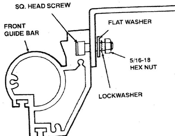
6. Holding the guide bar in place with one hand, insert a flat washer, lockwasher and nut on each screw starting from the center and alternating left and right. Finger tighten only until all six screws have washers, lockwashers and nuts installed. Hand tighten 4 nuts at saw table first. With a straight edge along the right side of the saw blade, align the blade aligning mark on the top of the front rail with the right side of the saw blade.
