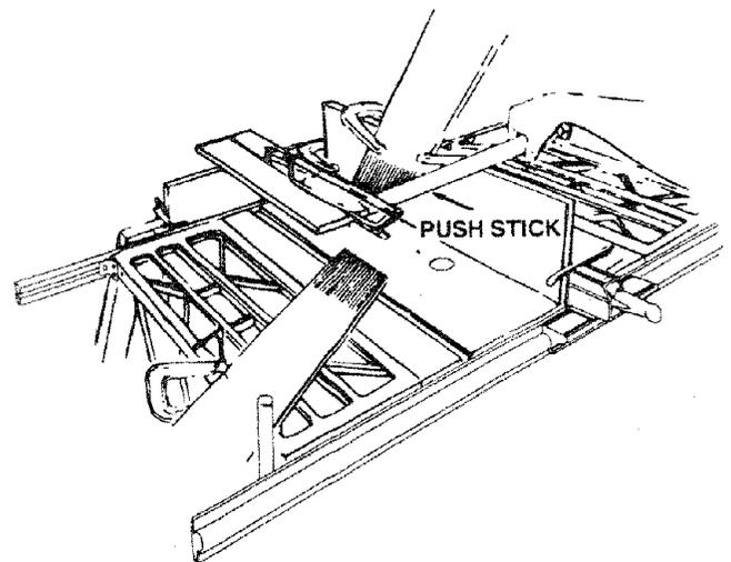
**WARNING: To avoid kickback push forward only on the part of the workpiece that will pass between the blade and the fence.**
