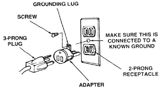
This plug requires a mating 3-conductor grounded type outlet as shown above.
