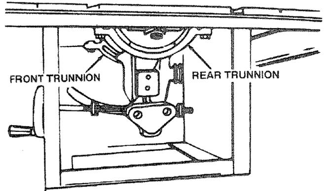
7. Loosen all three screws that hold the rear trunnion and all three screws that hold the front trunnion.
