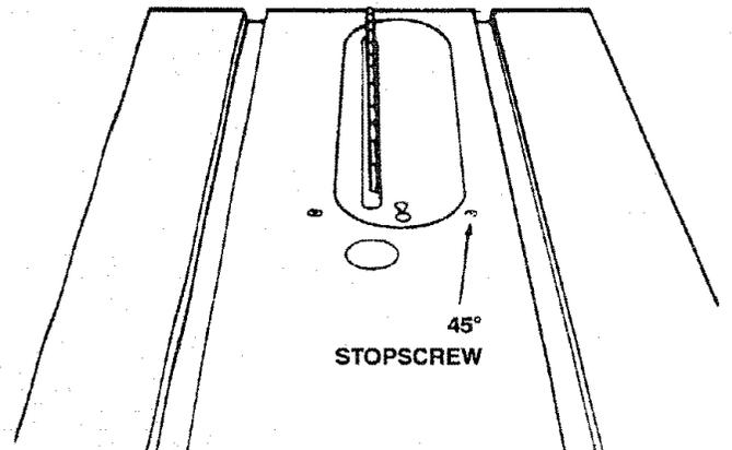
4. Loosen two screws on scale and adjust scale until POINTER points to 45 degree mark.
