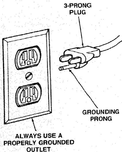
**WARNING: To avoid electrical shock, do not permit fingers to touch the terminals of the plug, when installing or removing the plug to or from the outlet.**
