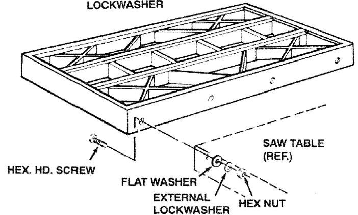
5. Line up front edge of extension with front edge of table. Line up top surface of extension with top surface of table at the locations indicated by the "X"s (see illustration).
