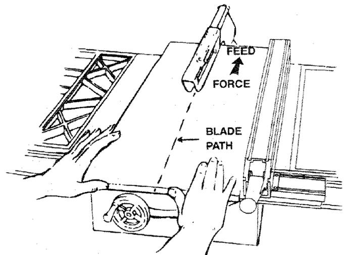
When "WIDTH OF RIP" is 2 in. or wider, USE THE PUSH STICK to finish pushing the work all the way past the blade.
