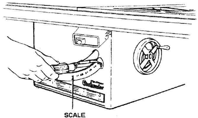
If blade is NOT 45° TO TABLE...STOP SCREW and SCALE must be ADJUSTED.
