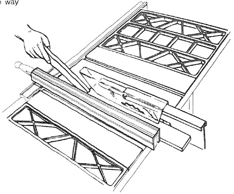
When WIDTH OF RIP is 1/2" to 2 in., the push stick CANNOT be used because the guard will interfere. USE the AUXILIARY FENCE/WORK SUPPORT and PUSH BLOCK.
