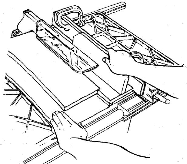
Narrow strips thicker than the Auxiliary Fence/Work Support may enter the guard and strike the baffle. CAREFULLY raise guard only enough to clear the workpiece. Use PUSH BLOCK to complete cut.
