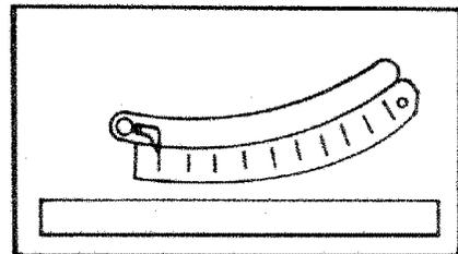
If blade is NOT SQUARE to table...the 90 degree stop screw must be ADJUSTED.
