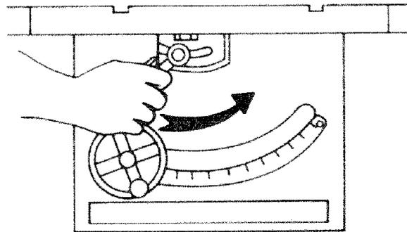
5. Blade should be square with table and pointer should point to "0".
