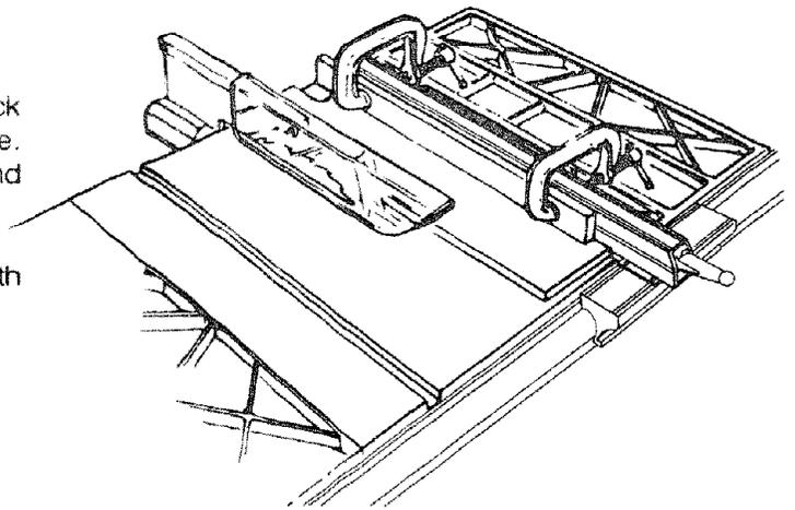
Feed the workpiece by hand along the AUXILIARY FENCE until the end is approx. 1 in. past the front edge of the table. Continue to feed using the PUSH BLOCK.
