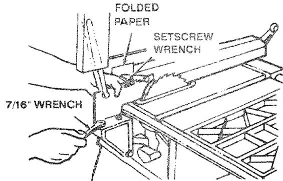
21. To remove BLADE GUARD AND SPREADER, loosen THUMBScrew...DO NOT LOOSEN OTHER SCREWS. This lets you remove and replace the guard without disturbing the spreader alignment.
