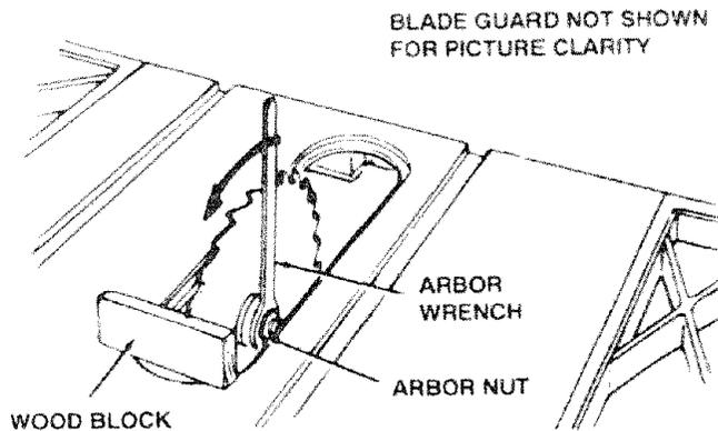
When installing the blade, make sure the teeth are pointing toward the front of the saw and that the blade and collars are clean, and free from any burrs. The HOLLOW side of the collar must be against the blade. Always tighten the arbor nut securely.
