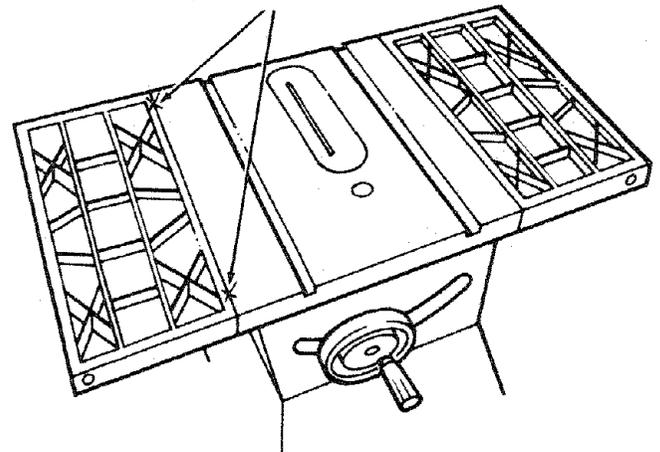
6. If adjustment is necessary (low in the center) use a "C" clamp to raise the center of the extension into position. Make sure front edge of extension is lined up with front edge of table. Then firmly tighten nuts.
