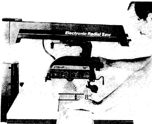
Fig. 147 - Hand Placement for Crosscuts
