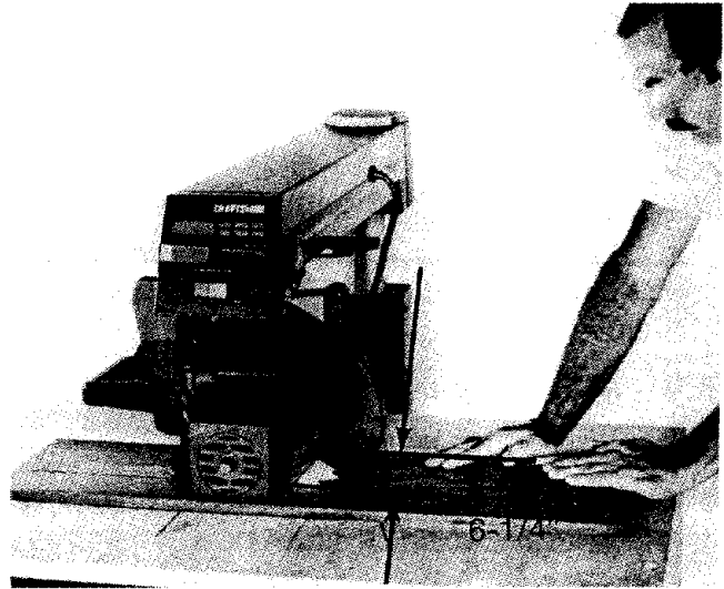
Fig. 158 Hand and Body Position for Making an In-Rip Cut
