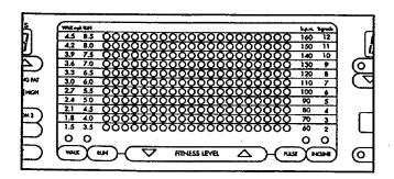
The settings of the first segment will be shown in the far left column, and the settings of the twentieth segment will be shown in the far right column. Red indicators will show the speed setting of each segment, and green indicators will show the incline setting of each segment.
