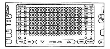
If you selected the WALK or RUN mode, red indicators will show the speed setting of each segment. If you selected the INCLINE mode, green indicators will show the incline setting of each segment. If you selected the WALK and INCLINE modes or the RUN and INCLINE modes, both red and green indicators will be lit.
