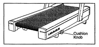
For a firmer cushion level, turn the knob clockwise; for a softer cushion level, turn the knob counterclockwise. Note: The faster you run on the treadmill, the firmer the cushion level should be. If the cushion level is too soft, the treadmill will bounce excessively.
