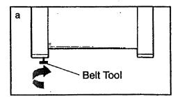
b. If the walking belt has shifted to the right, first remove the key and UNPLUG THE POWER CORD. Using the belt tool, turn the rear roller adjustment bolt counterclockwise 1/4 of a turn. Plug in the power cord, insert the key and run the treadmill for a few minutes. Repeat until the walking belt is centered.
