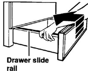
1. **Fit** ends of drawer slide rails into the drawer guides on both sides of opening.
