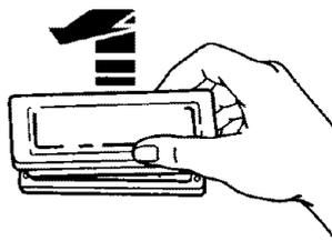
2. **Remove** glass light cover by grasping front edge of cover and pulling it away from the side wall of the oven.
