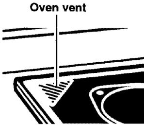
Hot air and moisture escape from the oven through a vent in the left rear corner of the cooktop. **Do not block the vent by using large pans or covers.** Poor baking/roasting can result.
