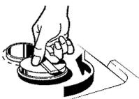
**NOTE:** To open detergent cup after it has been closed, unlatch the door. Press the **START/RESET** pad three times within two seconds and the detergent cup will release. A snapping sound may be heard.
