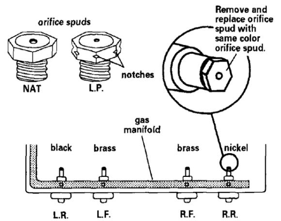
**5.** Locate Natural gas orifice spuds in literature package. Remove L.P. gas orifice spuds using a 3/8" combination wrench. Install Natural gas orifice spuds to replace the L.P. gas orifice spuds.
