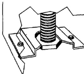
**7.** If installing the range in a mobile home, you MUST secure the range to the floor. Any method of securing the range is adequate as long as it conforms to the standards in the "Mobile home installation" instructions, Page 1.
