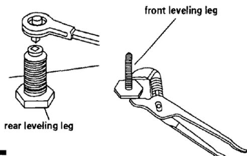
**5.** Remove cardboard shipping base from under range. Remove storage drawer. Use a 3/8" drive ratchet to lower rear leveling legs one-half turn. Use channel lock pliers to lower front leveling legs one-half turn.
