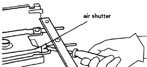
3. Using a flat-blade screwdriver, adjust the air shutter for each burner as needed. Close the air shutter to decrease the amount of air to the flame. Open the air shutter to increase the amount of air to the flame. Adjust the air shutter to the widest opening that will not cause the flame to lift or blow off of the burner.
