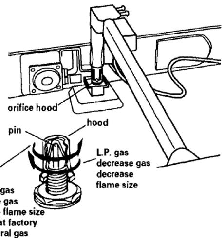
**6. Oven burner:** Use 1/2" combination wrench to loosen the orifice hood away from pin (approximately 2 to 2-1/2 turns). The burner flame cannot be properly adjusted if this conversion is not made.
