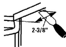
Carefully slide a putty knife in between the cooktop and the oven part of range. While gently lifting the cooktop, push in on the putty knife to release the clip. Repeat on other side.
