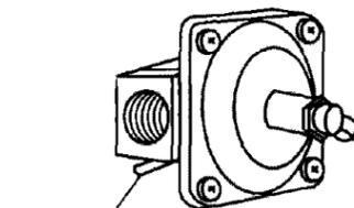
regulator shutoff valve in "on" position
