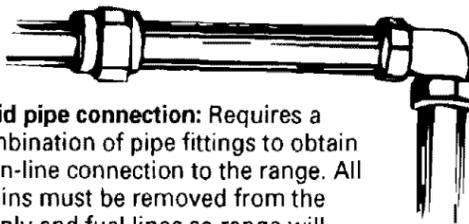
**Rigid pipe connection:** Requires a combination of pipe fittings to obtain an in-line connection to the range. All strains must be removed from the supply and fuel lines so range will be level and in line.
