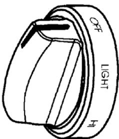
**15.** Push in and turn each surface unit control knob to "LIGHT" position. The flame should light within 4 seconds. Turn control knob to "HI" position after burner lights. **Do Not leave the knob in the "LIGHT" position after burner lights.**
