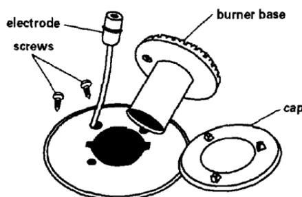
2. Remove storage drawer and oven racks. Remove burner grates, caps and screws holding burner bases to cooktop. Lift burners off cooktop.
