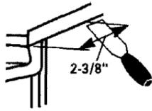
Carefully slide a putty knife in between the cooktop and the oven part of range. While gently lifting the cooktop, push in on the putty knife to release the clip. Repeat on other side.
