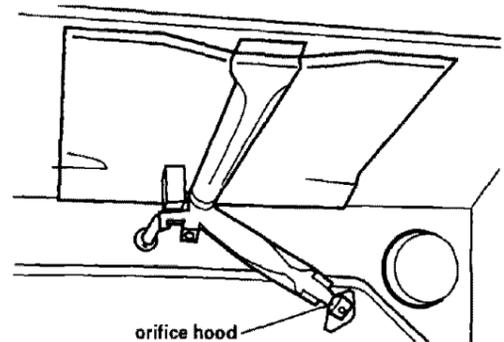
**7. Broil burner:** Use 1/2" combination wrench to loosen orifice hood away from pin (approximately 2 to 2-1/2 turns). The burner flame cannot be properly adjusted if this conversion is not made.
