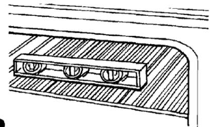
**8.** Place rack in oven. Place level on rack, first side to side; then front to back.
