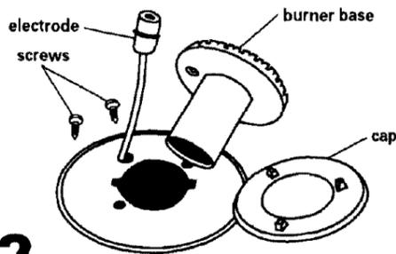
**2.** Remove storage drawer and oven racks. Remove burner grates, caps and screws holding burner bases to cooktop.
