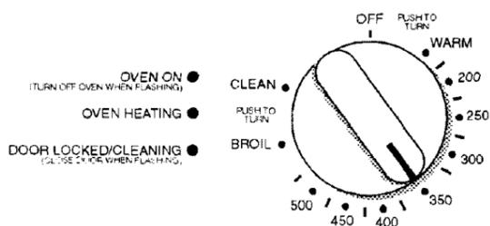
Push in and turn the oven selector control knob to "350°F." **The oven burner should light in 50-60 seconds; this delay is normal.** The oven valve requires a certain time before it will open and allow gas to flow.
