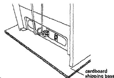
**3.** Keep cardboard shipping base under range to prevent damage to floor covering.
