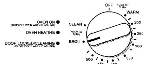
Push in and turn the oven selector control knob to "BROIL." **The broil burner should light in 50-60 seconds; this delay is normal.** The oven valve requires a certain time before it will open and allow gas to flow.
