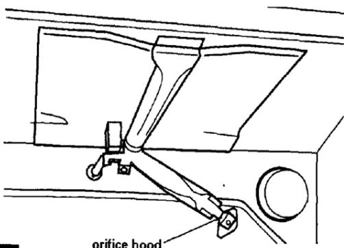
**7. Broil burner:** Use 1/2" combination wrench to turn the orifice hood down snug onto pin (approximately 2 to 2-1/2 turns). **DO NOT OVERTIGHTEN.** The burner flame cannot be properly adjusted if this conversion is not made.
