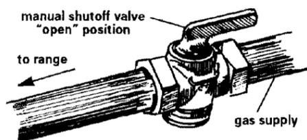
**11.** Check that range regulator shutoff valve is in the "on" position. Open the manual shutoff valve in the gas supply line. Wait a few minutes for gas to move through the gas line.
