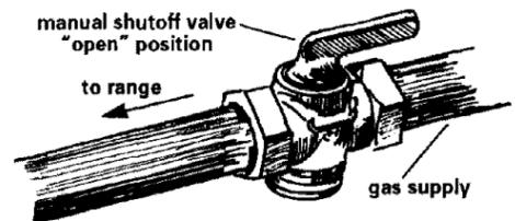
**Shutoff valve:** The supply line must be equipped with a manual shutoff valve. This valve should be located in the same room as the range and should be in a location that allows ease of opening and closing. The valve is for turning on or shutting off gas to the range. **Do Not block access to shutoff valve.**
