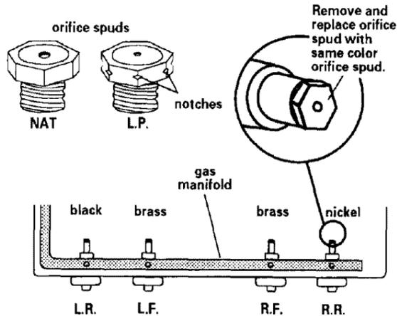
**5.** Prop open cooktop maintop. Remove the venturi plates. Locate L.P. gas orifice spuds in a literature package included with the range. Orifice spuds are color coded. Remove one Natural gas orifice spud at a time using a 3/8" combination wrench. Install the same color L.P. gas orifice spud to replace the Natural gas orifice spud.
