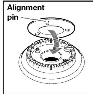
6. Turn on the burner to see if it will light. If the burner does not light after you have cleaned it, recheck cap alignment or contact an authorized service technician. Do not service the sealed burner yourself.
