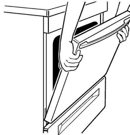
2. Rest the hinge hanger so that it is flat (at the bottom of the hinge hanger on the bottom of the front frame slot).
