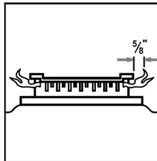
A good flame is blue in color. If the flames are uneven, you may need to clean the burner ports.
