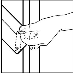
3. Rotate the door toward the range. Lift up the door until it stops. Do not use the door handle to lift the door. Rotate the door toward the floor and pull it toward you.
