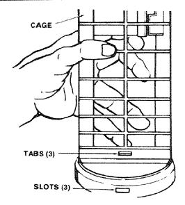
NOTE: If the cage needs to be removed, because the float is placed in the wrong way, use a slotted screwdriver and apply the slotted end to one of the cage tabs. Push in on the tab and lift the cage up. Tilt the cage slightly away from the open slot to release the other two tabs. Pull the cage away from the lid. To replace follow float cage assembly instructions.
