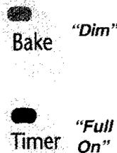
The display will show the operation for the pad with the “full on” indicator light. Press the function pad with the “dim” indicator light to recall that operation.
