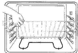
**TO REPLACE:** Place rack on the rack support in the oven; tilt the front end up slightly; slide rack back until it clears the lock-stop position; lower front and slide back into the oven.
