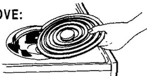
**TO REPLACE:** Insert element terminals into receptacle. Guide the element into place. Press down on the outer edge of element until it sits level on drip bowl.
