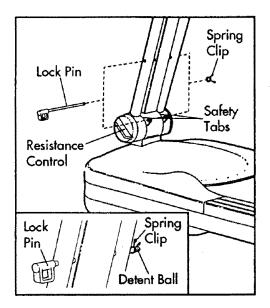
CAUTION: Always insert the lock pin through the safety tabs when using the upper body arms in the dual motion position. If you fall while exercising, the lock pin will limit the downward movement of the arms. When the lock pin is inserted through the safety tabs, do not lean on the upper body arms or the lock pin may be damaged. If the spring clip is not attached to the lock pin as instructed, the lock pin may slip out, resulting in injuring to the user.
