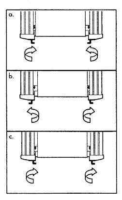
Before converting the CROSS WALK to the stowaway position, turn the resistance control (see the drawing on page 8) counterclockwise until the control turns freely. Next, unplug the power cord. Remove the lock knob and washer from the upright and lay the upright and the upper body arms on the walking belt. Keep the lock knob and washer in a secure location.
