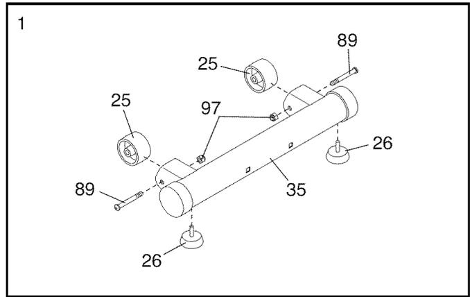
2. Have a second person tip the Frame (2) backward. Attach the Front Stabilizer (35) to the Frame with two M10 x 78mm Patch Screws (90).
