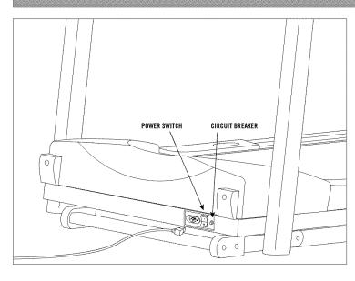
Connect power plug to the treadmill and connect the cord to a power outlet. The on/off switch is located next to the power cord. Flip this switch to the 'ON' position, so that the switch is lit. You will hear a beep and the console will light up.
